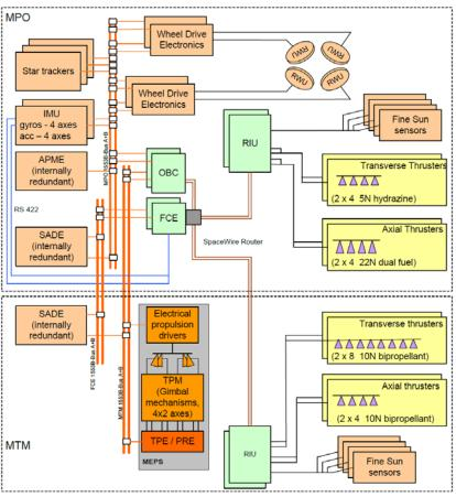
Figure 5: AOCS hardware architecture.
