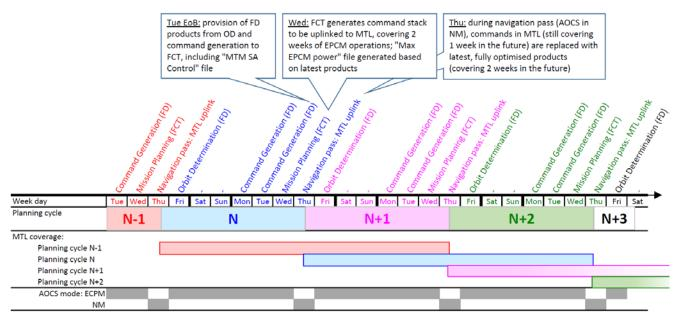
Figure 15: Weekly planning cycle during Electric Propulsion thrust arcs, including special processing for determining the MTM solar array pointing and the corresponding power available for EP thrusting.
