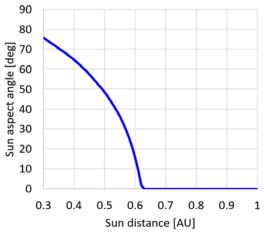
Figure 14: MTM solar array allowed Sun aspect angle depending on Sun distance (SAA of 0 deg means MTM SA is facing the Sun).
