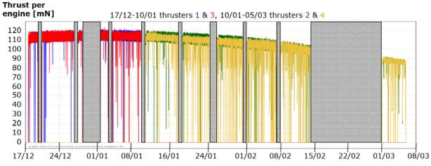
Figure 12: Thrusters and thrust levels used during the SEP1 arc. Greyed out periods indicate when the thrusters were OFF (S/C in NM). The large period before the last few days of thrusting in early March was to do an orbit determination with full accuracy prior to performing the final touch up manoeuvre of the arc.
