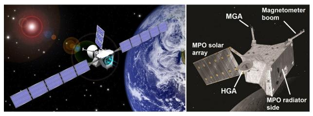
Figure 3: BepiColombo in cruise configuration (left), MPO at Mercury (right).
