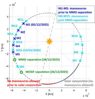
Figure 10: Mercury Orbit Insertion (MOI) sequence (depicted in ecliptic J2000 frame).
