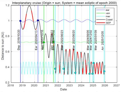
Figure 1: BepiColombo cruise trajectory, showing Sun distance, electric propulsion usage ("SEP"), and planetary flybys (at Earth, Venus, Mercury).
