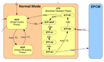
Figure 11: AOCS mode transitions for EPCM entry/exit.
