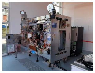
Figure 4: MPO element of the BepiColombo Engineering Test Bed (ETB) at ESOC.
