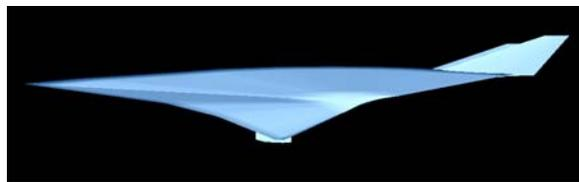
Fig. 3: Preliminary design of a Mach 8 cruiser based on a H<sub>2</sub> RBCC
