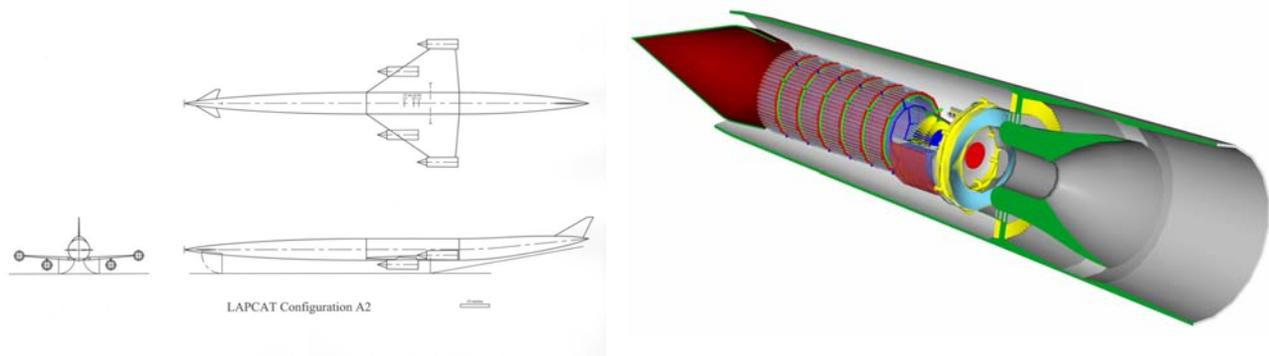
Fig. 1: LAPCAT A2: Mach 5 hydrogen based vehicle (left) with precooled turbofan-ramjet Scimitar engine (right)
