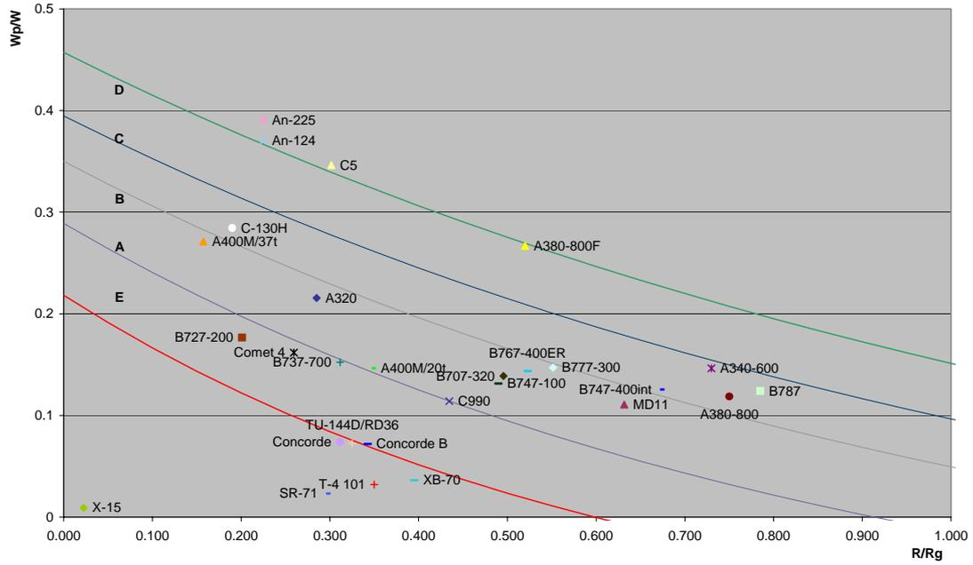
Fig. 1: Indicative payload fraction in function of non-dimensional range for various aircraft. Full lines A to E are based on eq. (4) for structural, propulsion & aerodynamic parameter variation.
