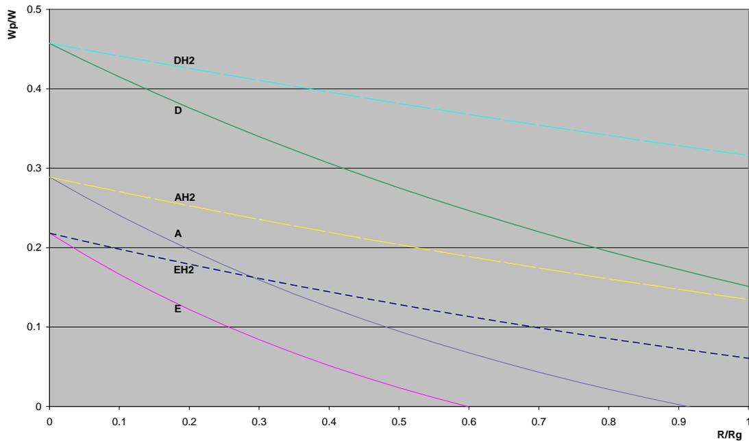
Fig. 2: Payload fraction dependence on fuel type: kerosene (full), hydrogen (dashed).
