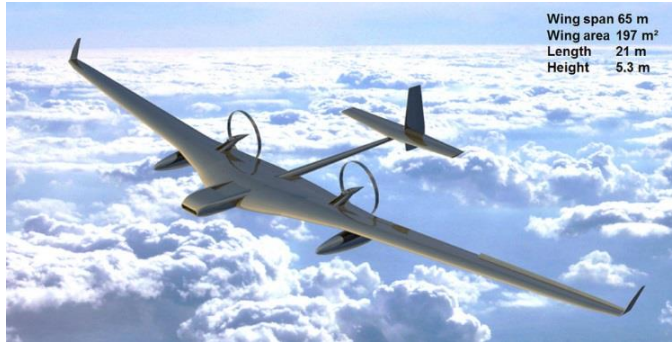
Figure 1: Project "StratoStreamer" HAPS aircraft by Leichtwerk AG [1]
