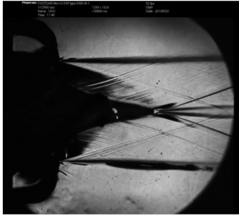
Fig. 1 Schlieren picture of a nearly adapted flow at NPR=45
