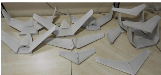
a) Illustration of the tail shapes manufactured for the Wind tunnel test campaign
