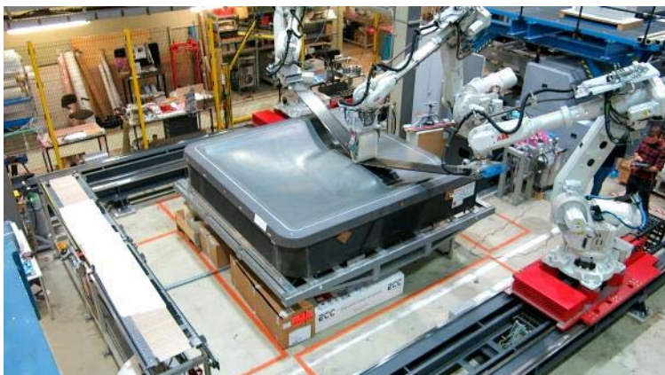
Fig. 2: Advanced Ply Placement (APP)
