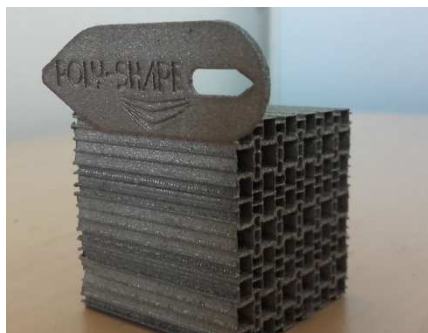
Print of an auxetic material Negative Poisson's ratio
