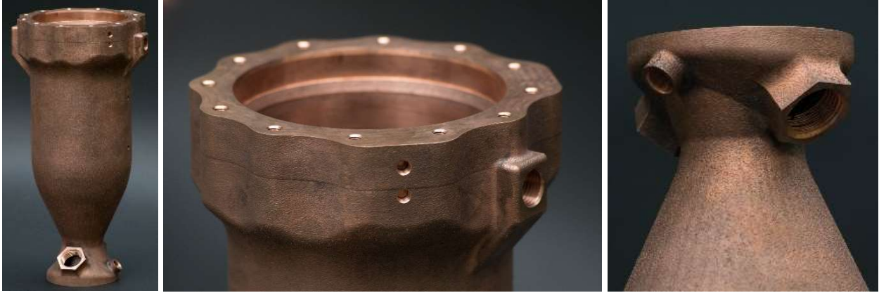
Figure 7: Arrax engine after manufacturing
