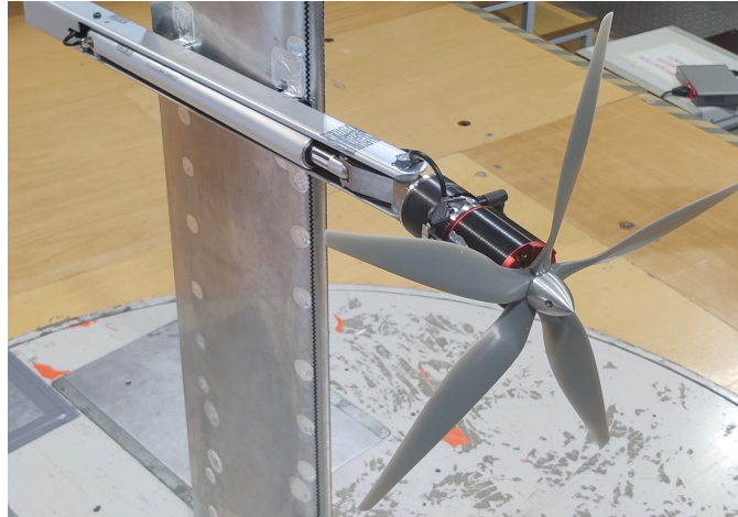
Figure 5: Detail view of pylon assembly showing support structure, linear actuator, six-component load cell, motor and 5 bladed 18x10 propeller.
