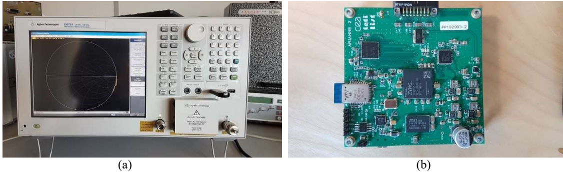
Figure 5: TDR measurement tools: (a) a Vector Network Analyser (VNA) , (b) CEA TDR sensor.
