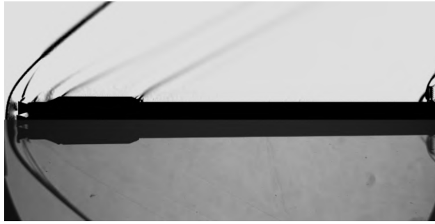
Figure 5: Schlieren photograph comparison for Mach 2 baseline case
