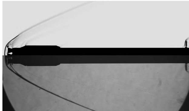
Figure 11: Schlieren photograph comparison for Mach 3.6 baseline case
