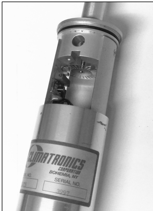
Figure 1: (Left) Opto-electronic output signal generator system of the Climatronics 100075 cup anemometer. (Right) Examples of sampling the analog square-wave output signal of a cup anemometer with the same sampling frequency at different wind speeds. The output voltage y is plotted in relation to the non-dimensional time t \cdot f (where f is the anemometer's output frequency). From [27].
