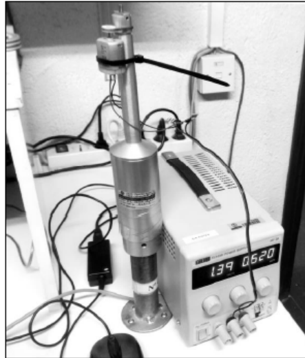
Figure 2: Testing set-up for measuring the Climatronics 100075 cup anemometer signature in still air.
