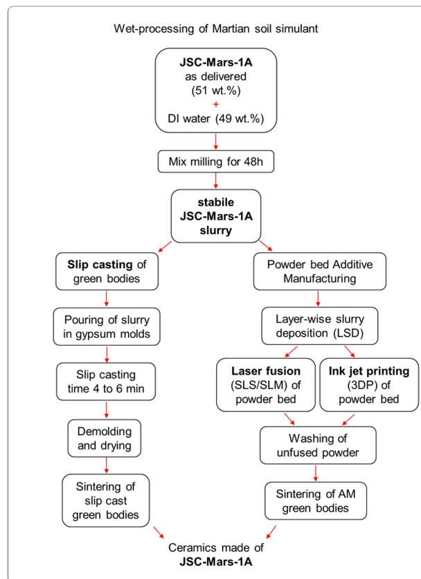
Figure 2: Possible wet-processing routes for JSC-Mars-1A slurry. This paper presents results for slip casting and LSD using laser fusion of the resulting powder bed.
