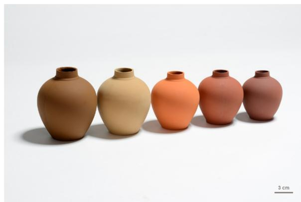
Figure 1: Ceramics made by slip casting of JSC-Mars-1A slurries. The image shows the same geometry after different heat treatments - from left to right: directly after demolding, dried green body, sintered at 1000°C without dwell time, 1130°C without dwell time, 1130°C with 10 hours dwell time.
