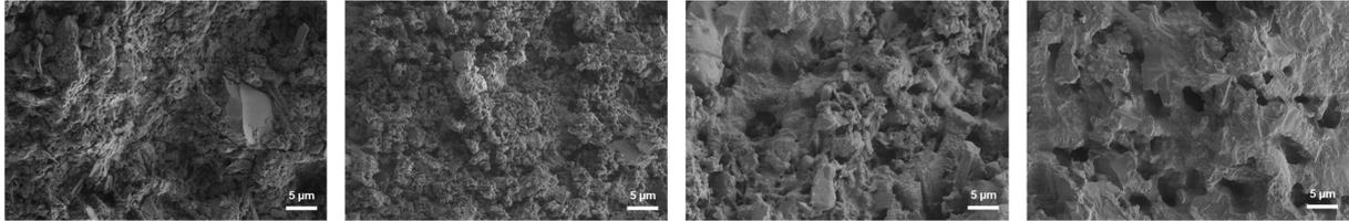
Figure 4: SEM micrography of obtained microstructure. From left to right: (a) green body, (b)  $1000^\circ\text{C}$  without dwell time, (c)  $1130^\circ\text{C}$  without dwell time, (d)  $1130^\circ\text{C}$  with 10 hours dwell time.
