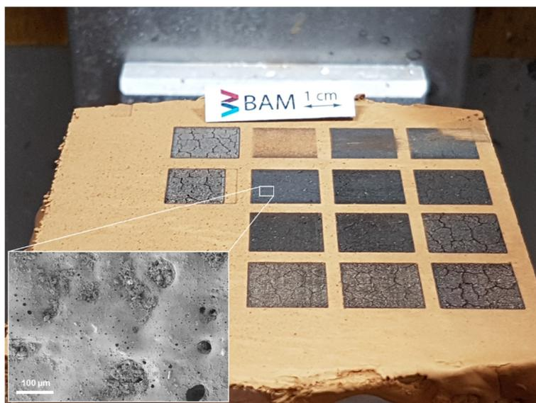
Figure 5: Layer-wise slurry deposition of JSC-Mars-1A. The powder bed was selectively fused using a laser.
