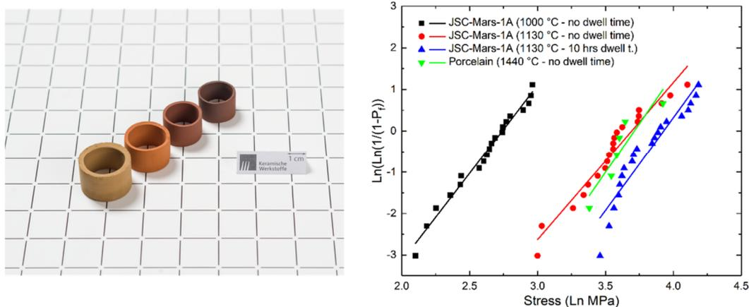
Figure 3: Slip cast JSC-Mars-1A ring test geometries and Weibull probability of failure plot for the three sintered rings and a porcelain reference.
