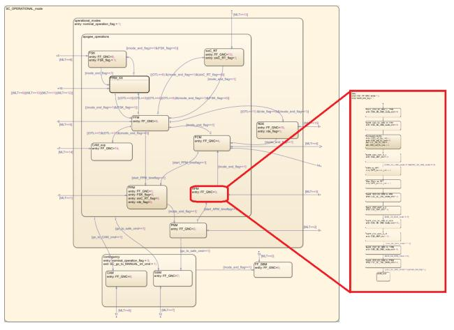
Figure 8: Example of the transition logic for the different FF-GNC modes when in OPERATIONAL mode. Each one of the boxes correspond to a different FF-GNC mode and its associated flight plan
