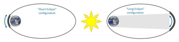
Figure 2: Different type of eclipses existing for high elliptically orbits
