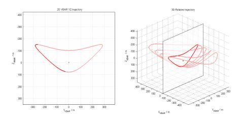
Figure 4: Shape of the relative trajectory described when SC are in Proba-3's Safe orbit (by courtesy of GMV)
