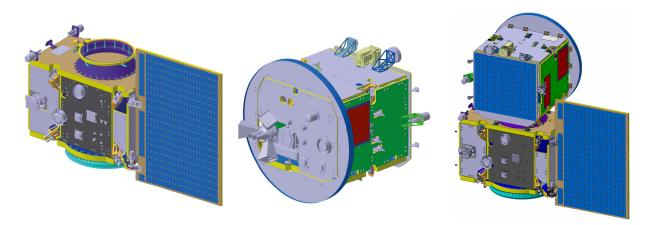
Figure 1: External view of the Coronagraph spacecraft (CSC, left), the Occulter spacecraft (OSC, center), and both SC in STACK configuration (right)
