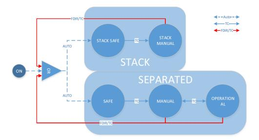
Figure 6: SC modes defined for Proba-3. Different modes exist depending on the SC being in STACK or separated
