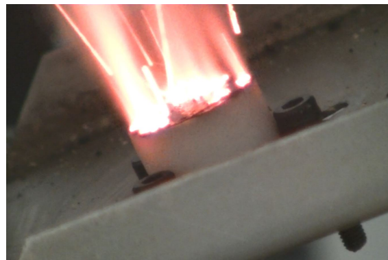
(b) Instantaneous ignition (P1) across a large part of the irradiated surface.
