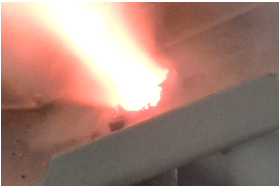
(c) Coarse Propellant flame structure with a more turbulent luminous flame showing uneven regression at the sample edge.
