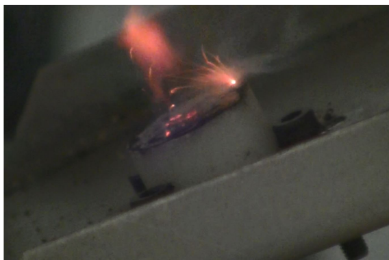
(a) Ignition of the coating (P2) showing ignition to start below the irradiated surface.
