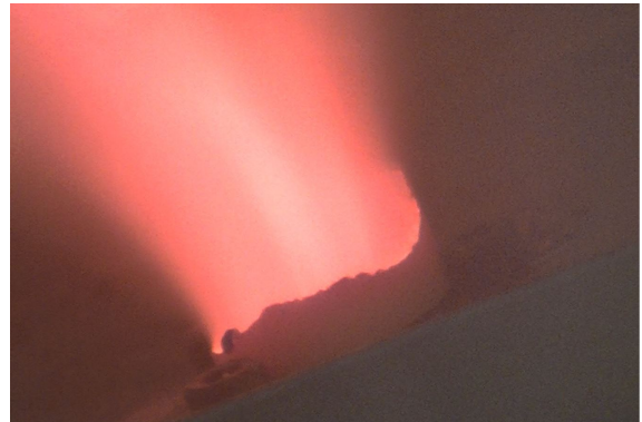
(d) Fine propellant showing more even regression with a smooth edge at which combustion occurs.
