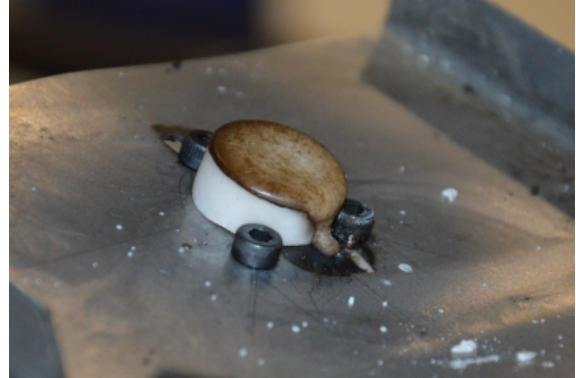
(b) Extinguished propellant (no 12) sample with molten propellant surface.
