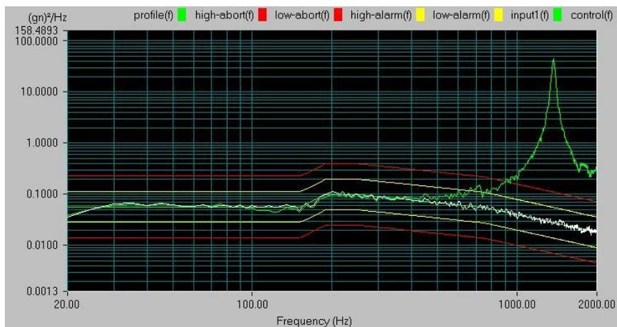
Figure 11: Random vibrations response for X axis
