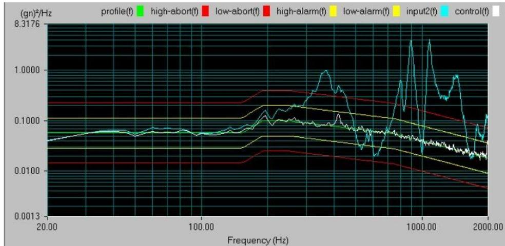
Figure 12: Random vibrations response for X axis
