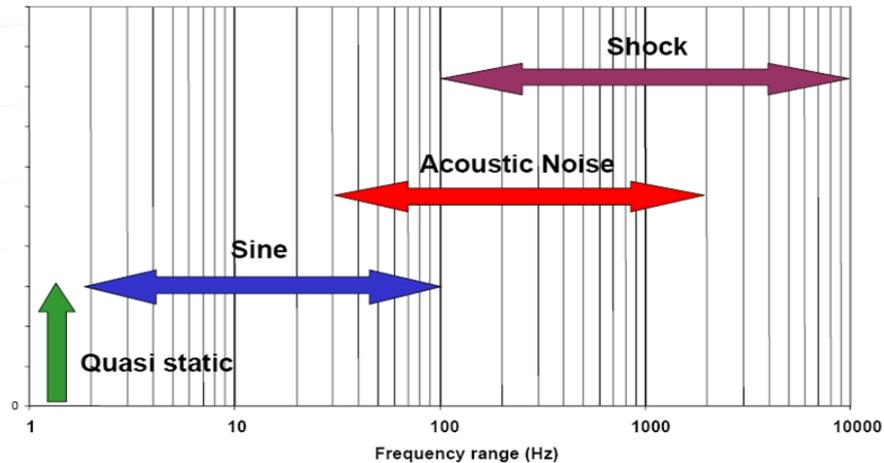
Figure 1: Static and dynamic environment specification according to [3]
