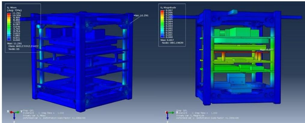
Figure 7: The stress and deflection in the Y-axis
