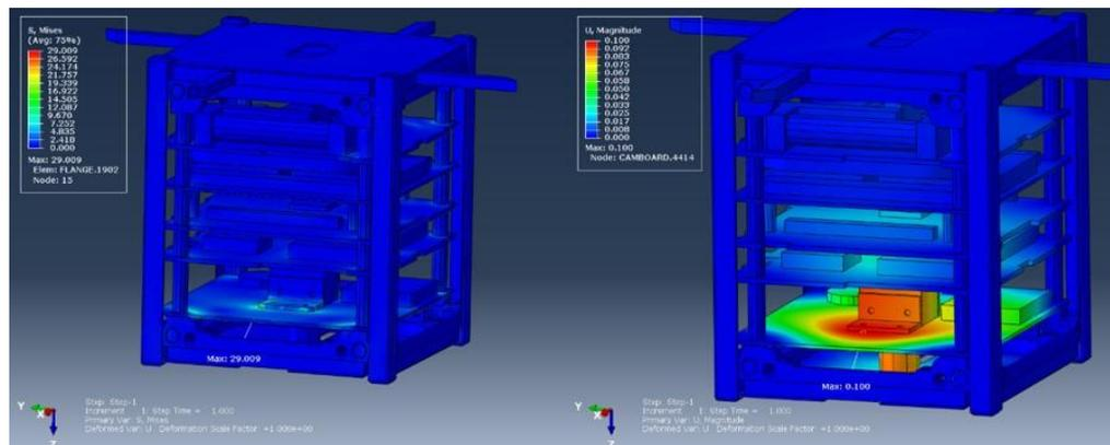
Figure 8: The stress and deflection in the Z-axis
