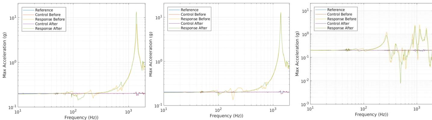
Figure 9: Low-level sine sweep response for X, Y and Z axes (left to right)
