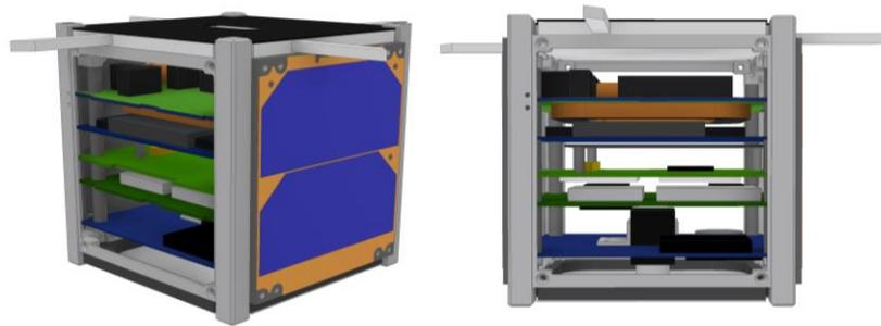
Figure 3: Simplified 3D model of MYSAT-1 used for FEA simulations
