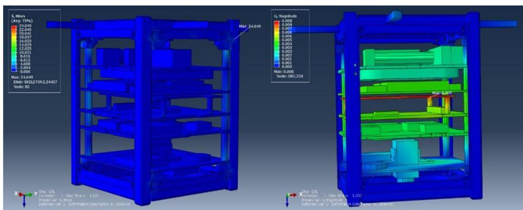
Figure 6: The stress and deflection in the X-axis
