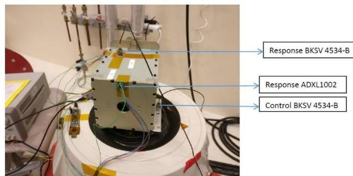
Figure 5: MYSAT-1 test set-up (X and Y directions)
