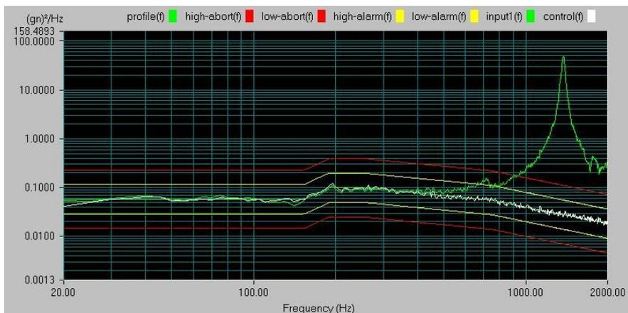
Figure 10: Random vibrations response for X axis
