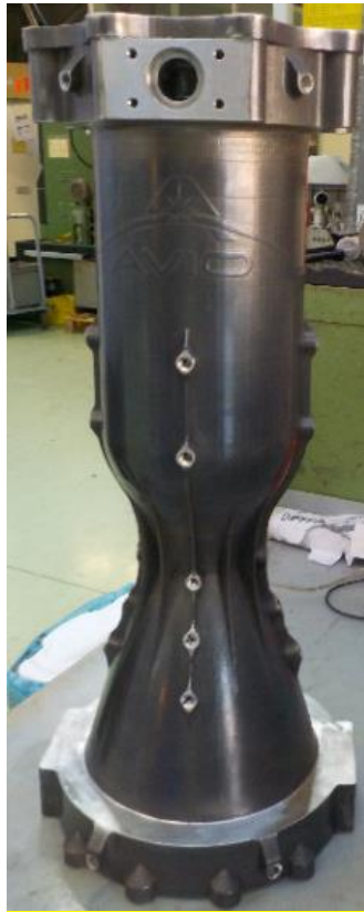
Figure 4 – Sub-scale TCA for development testing.
