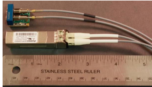
Figure 9. Size comparison of Glenair 2-fiber transceiver with commercial datacom SFP pluggable transceiver.
