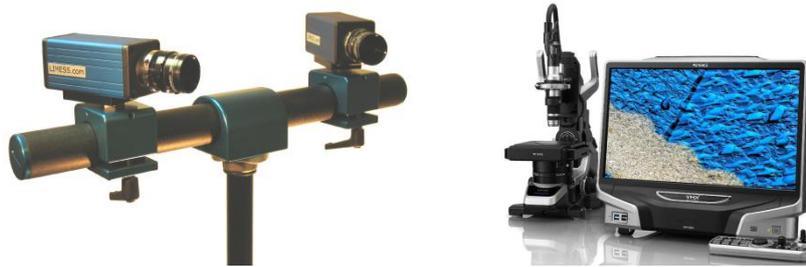
Figure 5: Devices for the measurement of the deformation of the TMF panel during the TMF test: stereo camera system (left) and after the TMF test: digital microscope (right)
