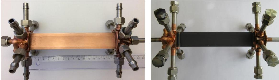
Figure 7: The liquid booster nozzle throat TMF panel made from CuCrZr in the laser-loading section (left) and coated TMF panel (right)
