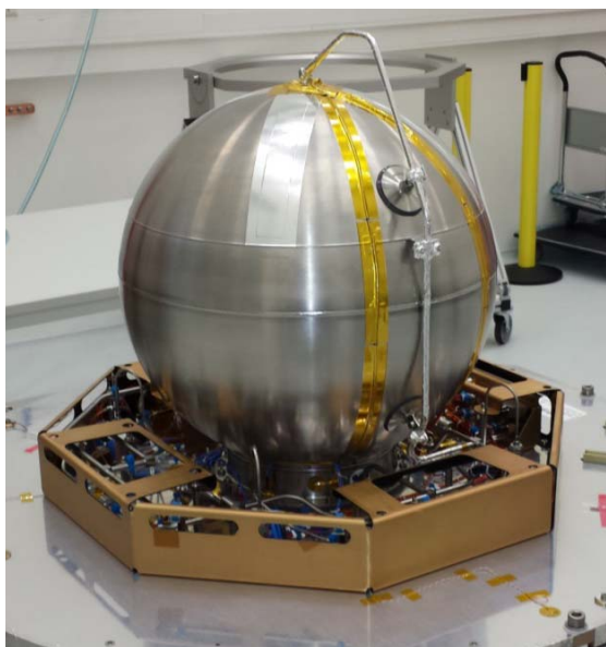
Figure 4 MYRIADE satellite propulsion subsystem for Hydrazine and LMP-103S
