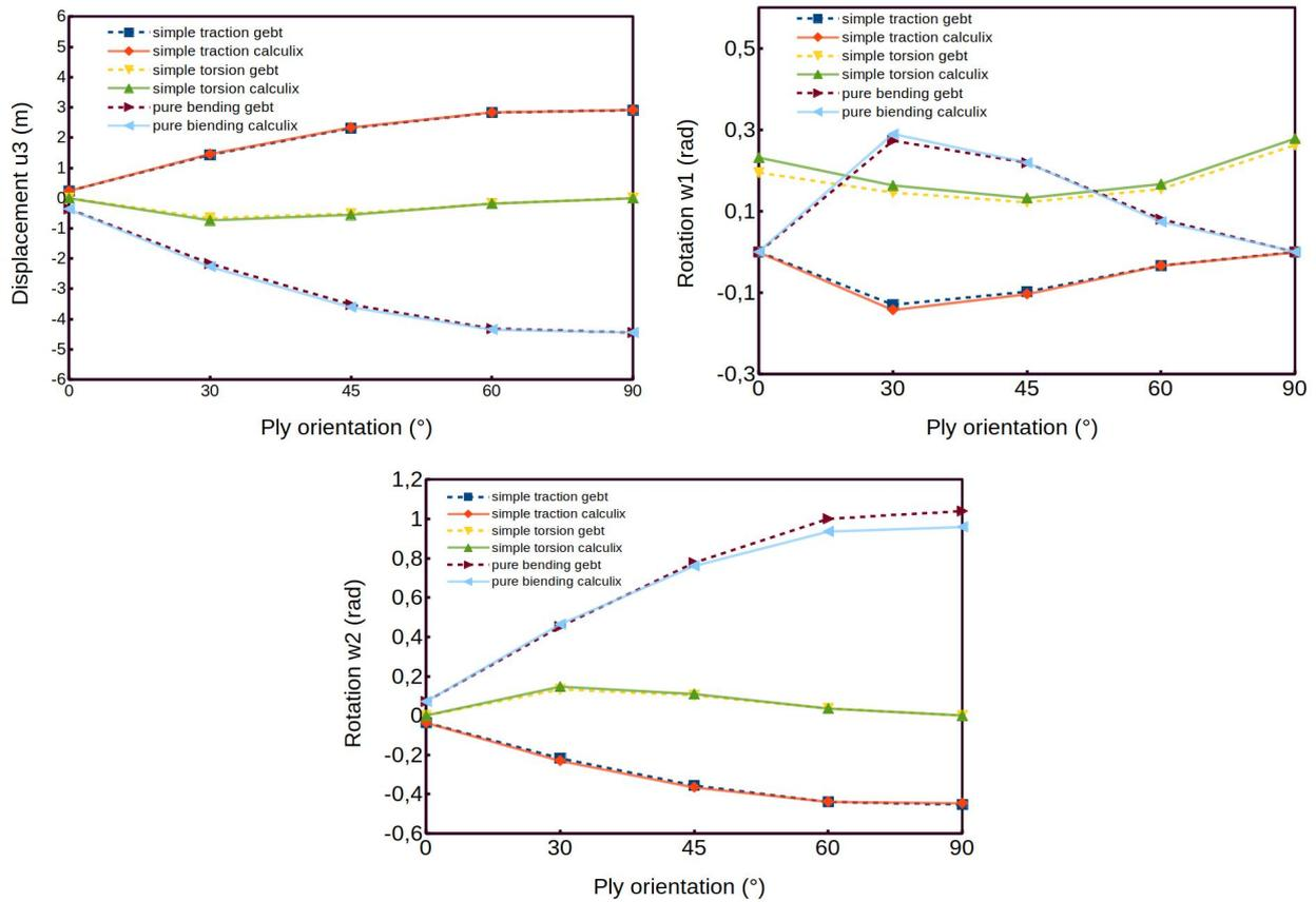
Figure 4: Comparison between GEBT computation code and Calculix results
