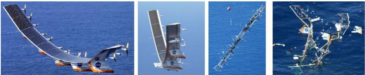
Figure 1: Wreckage of Helios on the 26th June 2003<sup>3</sup>
