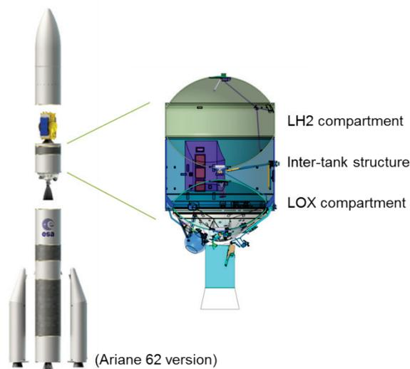
Figure 1: Ariane 6 launcher with upper propulsion module.
