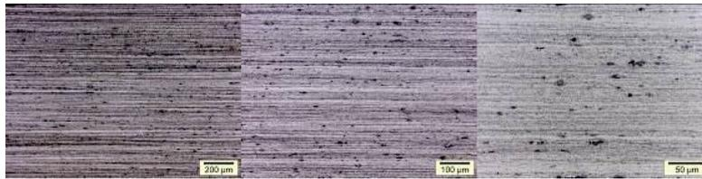
Figure 5: Metallographic analysis in rolling direction (L).
