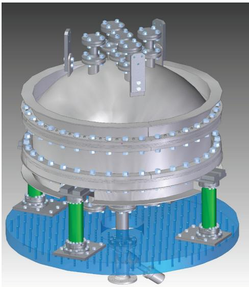
a) AlMgSc-Tank mounted on the mounting plate
