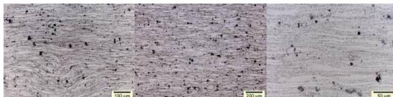
Figure 6: Metallographic analysis in perpendicular direction (LT).
