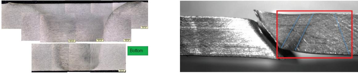
Figure 7: FSW microsections of 5028H116. The blue lines indicate the position of weld zone. Fracture started from the edge of the weld zone under an angle of 45° in direction of the base material.
