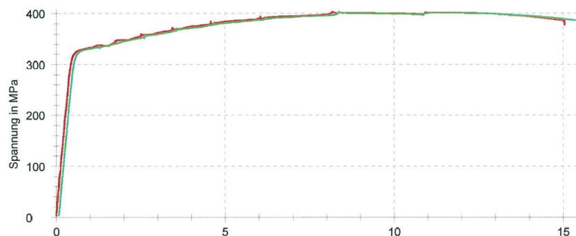
Figure 8: typical stress-strain curve of virgin base material (RED) and after H<sub>2</sub>O<sub>2</sub> four weeks exposure (GREEN).
