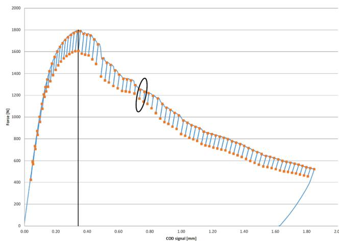
Figure 4: Typical force-COD curve at room temperature.
