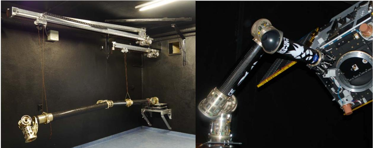
Figure 11: WMS1 LEMUR manipulator arm (left) and WMS2 manipulator for ORCO activity (right)
