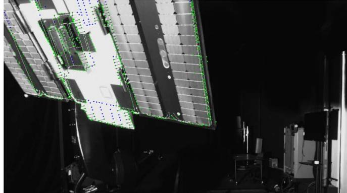
Figure 8: Poor edge tracking due to a textured surface
