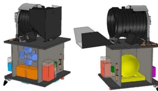
Fig. 7: SBSS platform with telescope (internal view)
