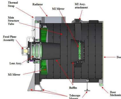
Figure 4: Strategy Cross section through the payload
