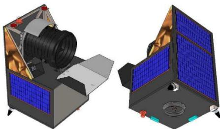
Fig. 6: SBSS platform with telescope (external view)
