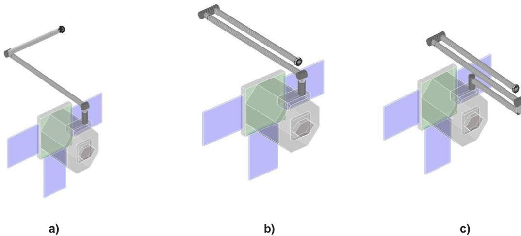
Figure 14: Robotic arm architectures
