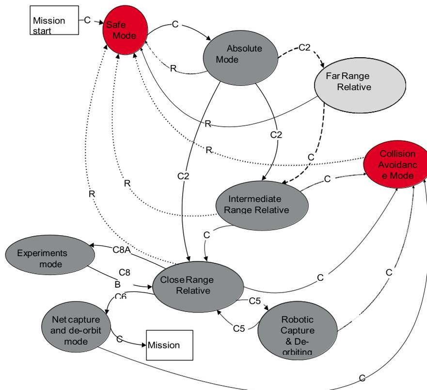
Figure 13: High-level GNC mode diagram
