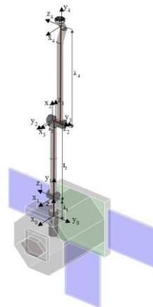
Fig. 15: Architecture „I1” and Denavit-Hartenberg coordinate systems
