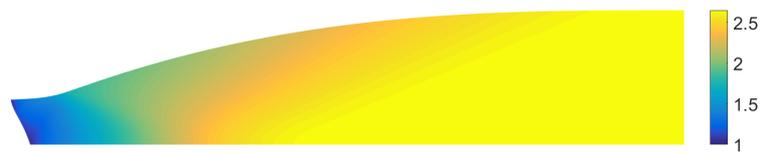
Figure 5: Mach number contourmap of the facility nozzle-IDG computed by MoC ( $M_0 = 3$ )
