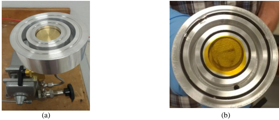
Figure 6: Vacuum wallet (a) before and (b) after loading of irradiated PI sample
