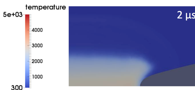
Figure 13: Temperature fields 2\mu s after the ignition beginning, starting with a stoichiometric propane-air mixture, and using the MECH_merged_33.
