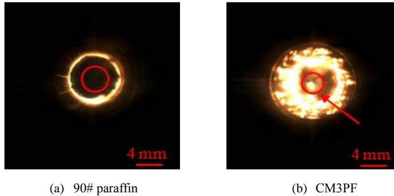
Figure 3: Combustion images of CM3PF and 90# pure paraffin at 3.5 s after ignition
