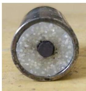
Figure 1: A CM3PF tested sample with the B/KNO<sub>3</sub> igniting charge
