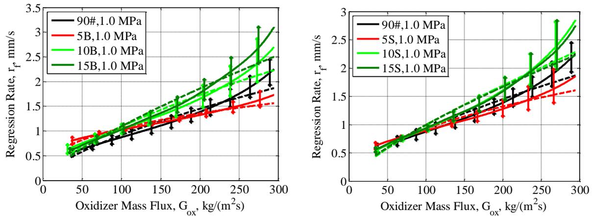
Figure 5: Regression rates of CM3PF at 5%, 10% and 15% granular polymer and 90# pure paraffin
