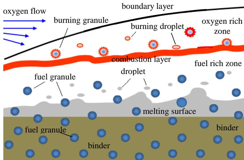
Figure 4: Disintegration process of CM3PF
