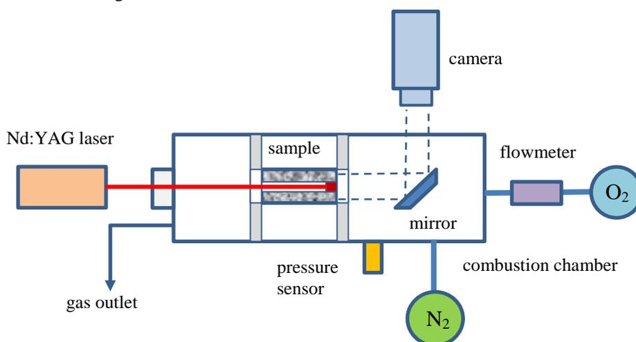
Figure 2: Experimental set to test regression rate of CM3PF
