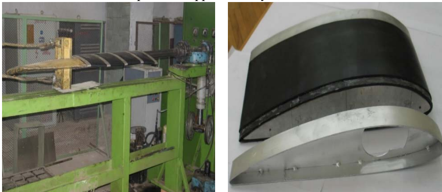
Fig.3. Stand for static tests and blade with flexible elements and rib.
