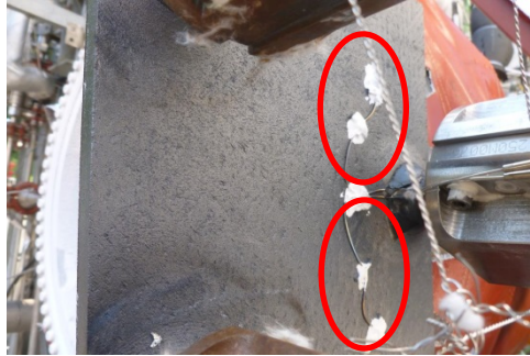
Figure 5. Thermocouples installed on the flap
