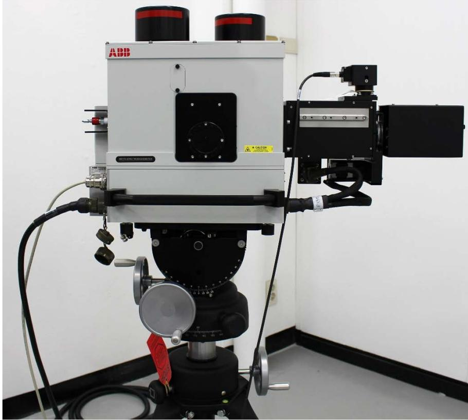
Figure 4: Spectroradiometer
