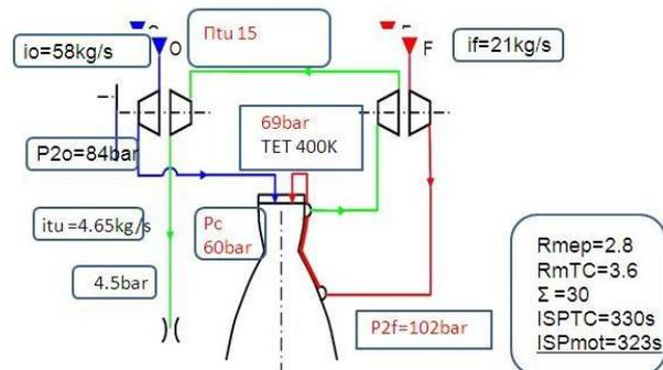
Figure 3: Preliminary design Bleed - LOX/CH<sub>4</sub> - 250 kN.
