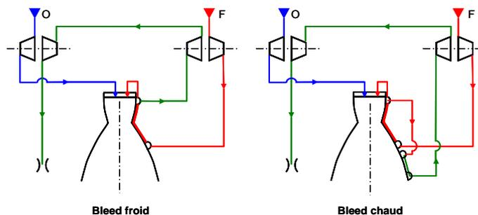
Figure 2: Cold bleed and hot bleed cycles engine.
