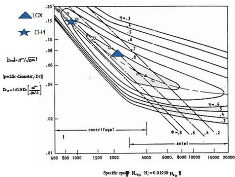
Figure 7: Representative Ns-Ds diagram for centrifugal and axial flow turbopumps.
