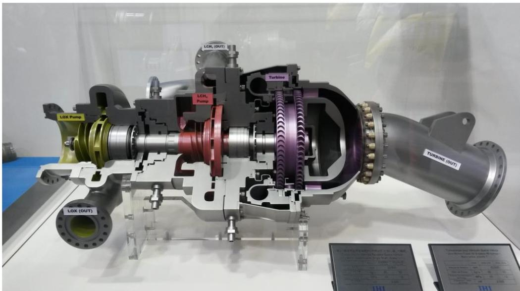
Figure 6: LOX/CH<sub>4</sub> single stage single shaft turbopump - Le Bourget 2015
