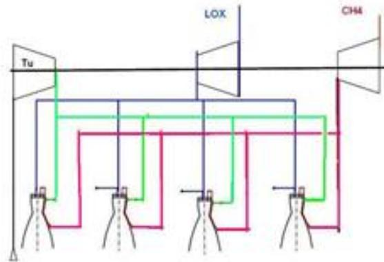
Figure 10: Four combustions chambers in propulsion bay
