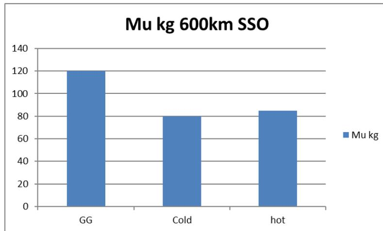
Figure 8: Engine cycle impact on payload mass
