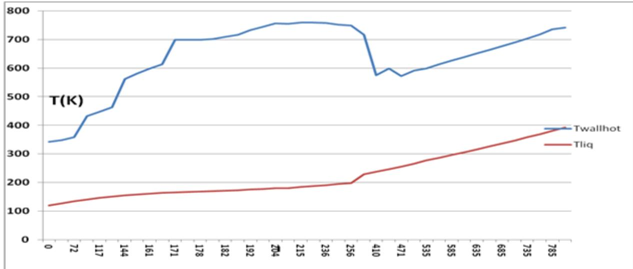
Figure 5: Hot wall gas temperature and methane liquid temperature.
