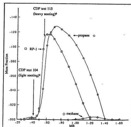
Figure 1: Soot mass fraction predictions vs MR for LOX/RP-1, Propane and Methane.  $P_c = 68 \text{ atm}$ .
