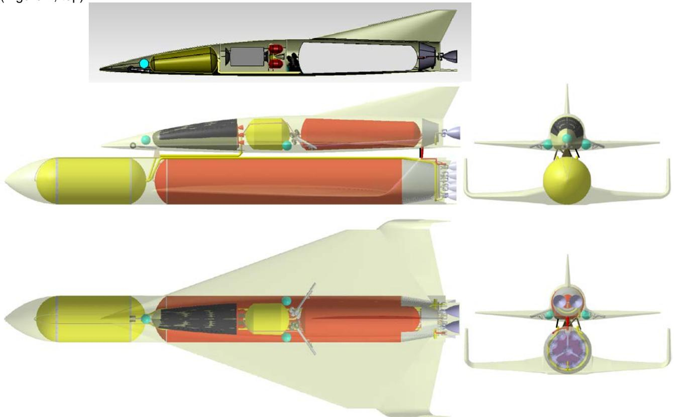
Figure 2: Sketch of SpaceLiner 7-3 launch configuration with passenger version (SLP) with its booster stage at bottom position and orbital stage of SLO in insert at top
