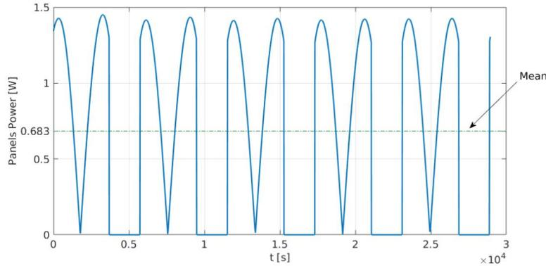
Figure 8: Available solar power in nominal pointing mode.
