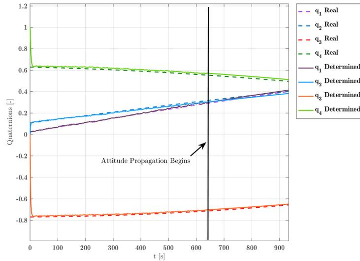
Figure 5: Attitude determination performances, starting from unknown attitude state in terms of quaternions  $\mathbf{q}$ . (All sensors are operational before the point highlighted by the vertical black line. Then the attitude is propagated because the spacecraft enters in eclipse).
