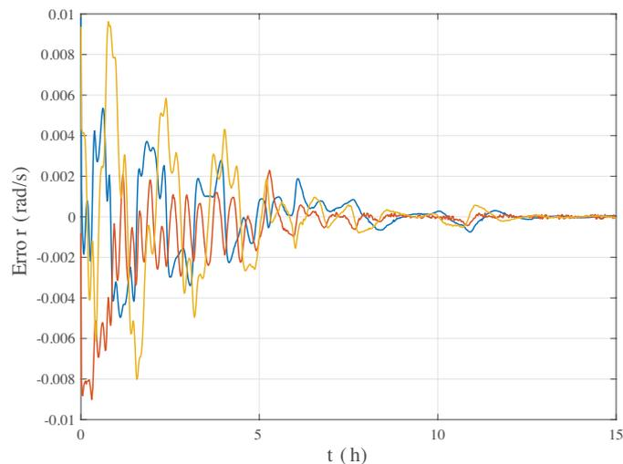
Figure 3: De-tumbling phase: error with respect to the nominal angular velocity.
