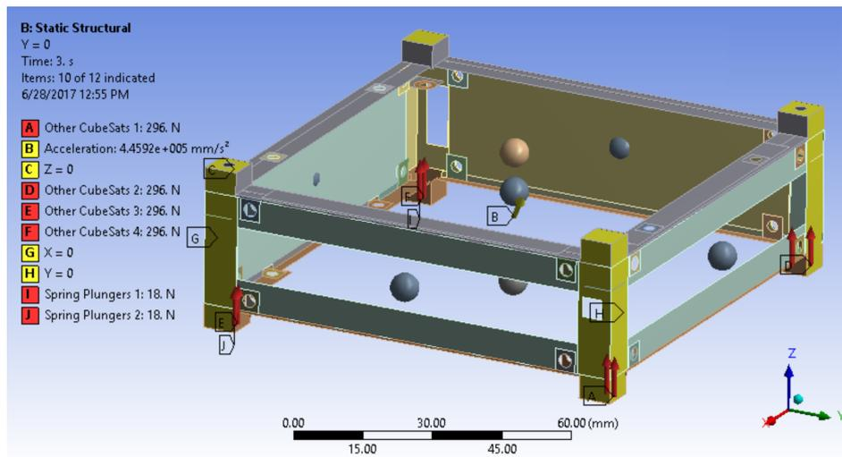
Figure 10: Shell model of FEES structure with applied loads and boundary conditions.
