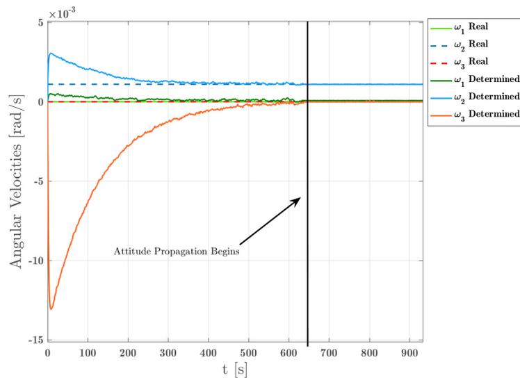
Figure 6: Angular velocities determination performances, starting from unknown angular velocity  $\omega$ . (Simulation related to the one presented in fig. 5. All the details in the relative caption).
