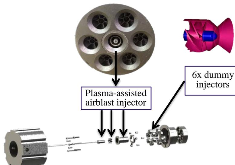
*fig-1 plasma-assisted seven point LDI Combustor*
