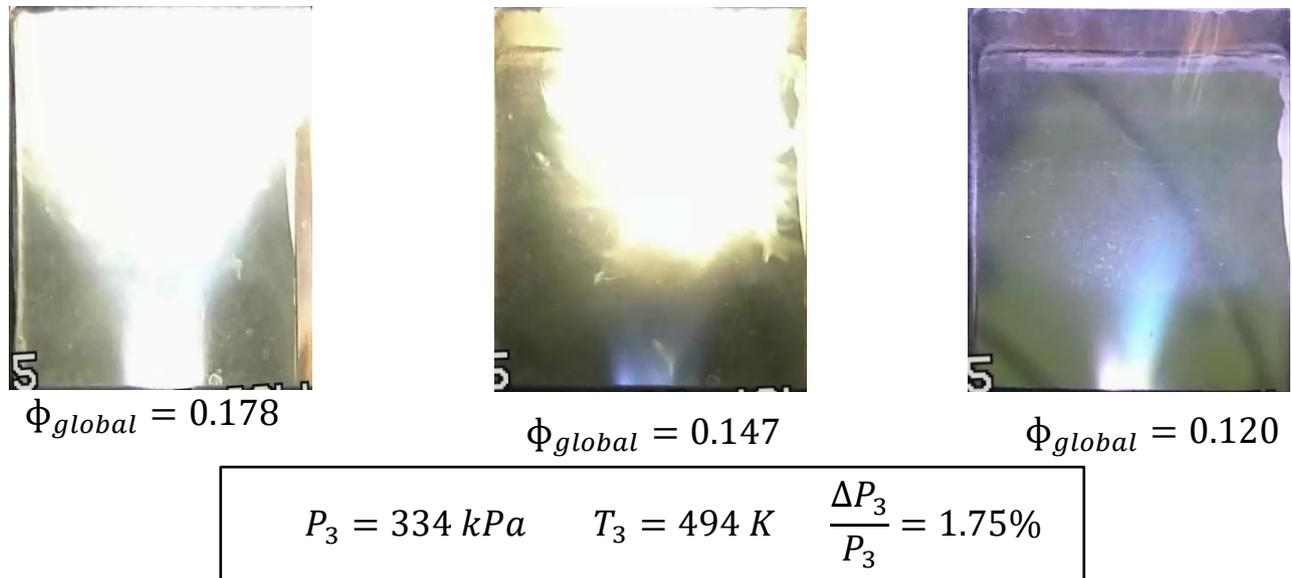
fig-3 Sequential images of plasma-assisted flame at decreasing equivalence ratio
