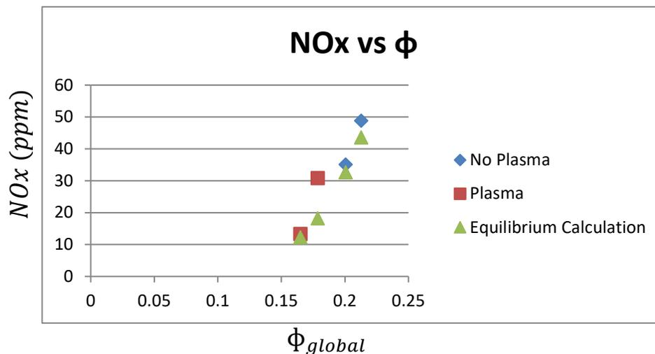
fig-4 Plot of NOx emissions as a function of global equivalence ratio
