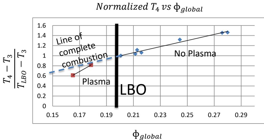
*fig-2 Plot of reduced temperature vs equivalence ratio to show lean limit extension*
