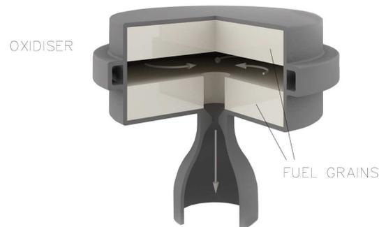
Figure 1: Vortex flow pancake hybrid rocket engine
