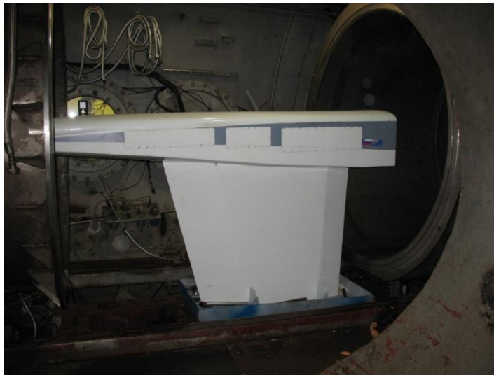
Fig. 3. Stand module HEXAFLY-INT on the dynamometer platform of the high stand Table 1 shows the test results.
