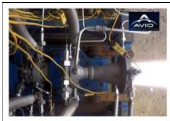
Figure 10: Hot firing test of ALM injector head
