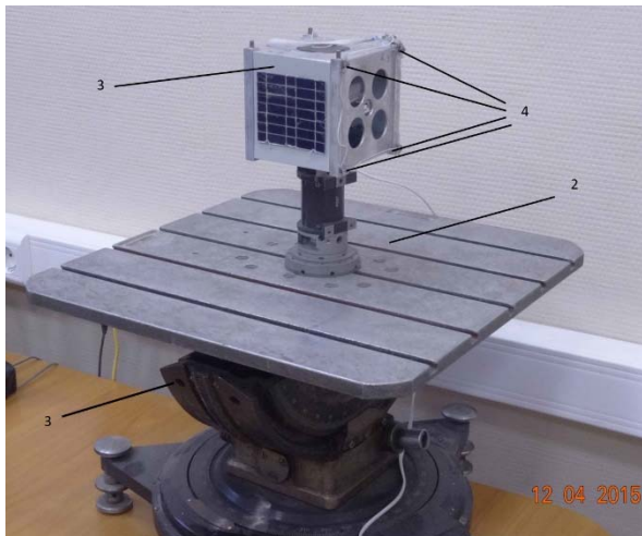
Figure 1: Stand for the experimental investigation of the optical system relative orientation picosatellites (CubeSat)
