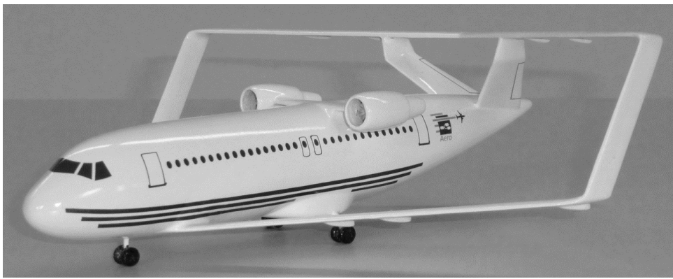
Figure 1: Box wing aircraft model developed by AERO - Hamburg University of Applied Sciences. [2]
