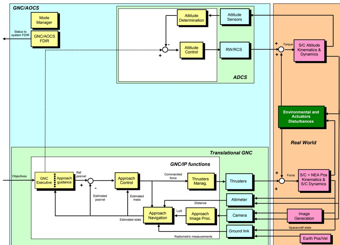
Figure 3: Functional architecture during Close Approach (IPM, ATPM, TPM)
