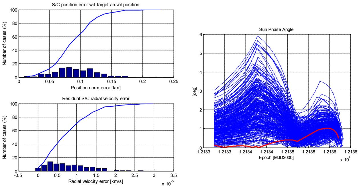
Figure 6: Close Approach arrival position and velocity errors statistics (left), and sun phase angle (right), in Monte Carlo simulation
