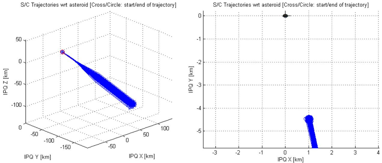
Figure 5: Close Approach trajectories in Monte Carlo simulation (left: full-scale // right: zoomed at arrival)
