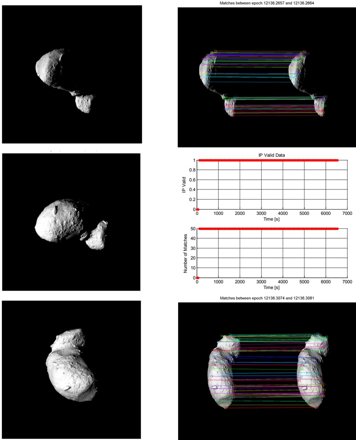
Figure 14: Body-Fixed Hovering camera images (left, selected 3 of 109) (courtesy of ADS-F) and FDT results (right, selected 2 consecutive image pairs and status in overall durations)
