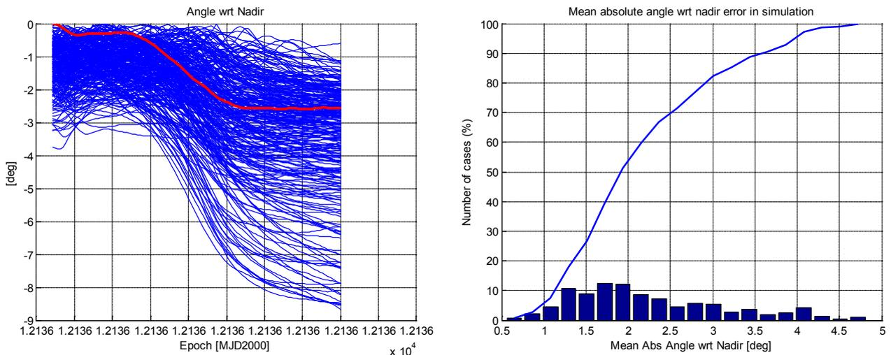
Figure 12: Body-Fixed Hovering angle wrt nadir (left) and mean angle statistics (right) in Monte Carlo simulation
