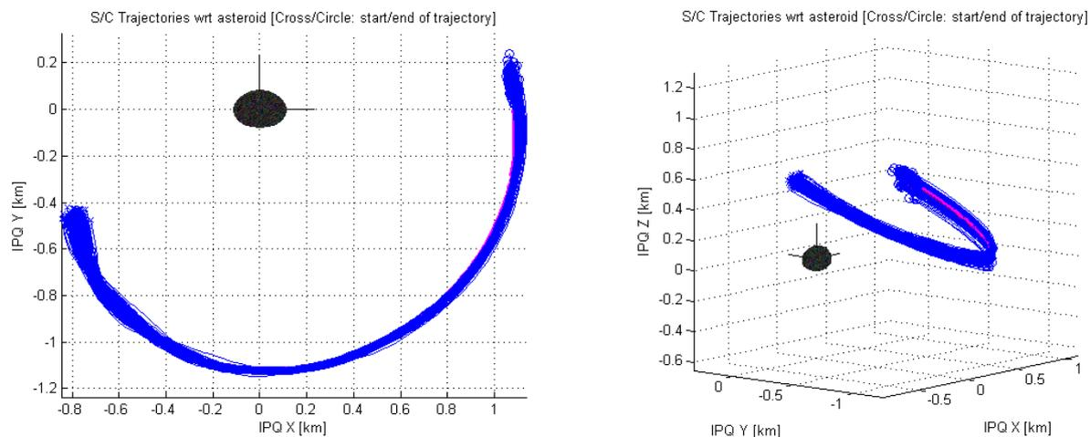
Figure 11: Body-Fixed Hovering trajectories in Monte Carlo simulation (left: X-Y // right: 3-axis view)
