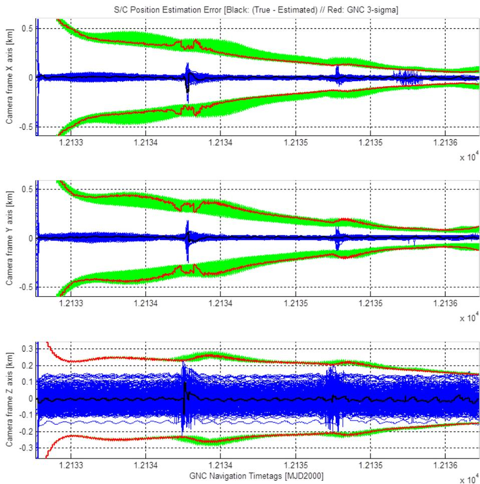
Figure 8: Close Approach navigation relative position estimation errors in Monte Carlo simulation (black-blue: error in all cases // red-green: filter 3-sigma knowledge in all cases)
