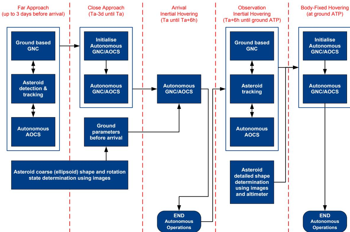
Figure 1: GNC/AOCS operations concept
