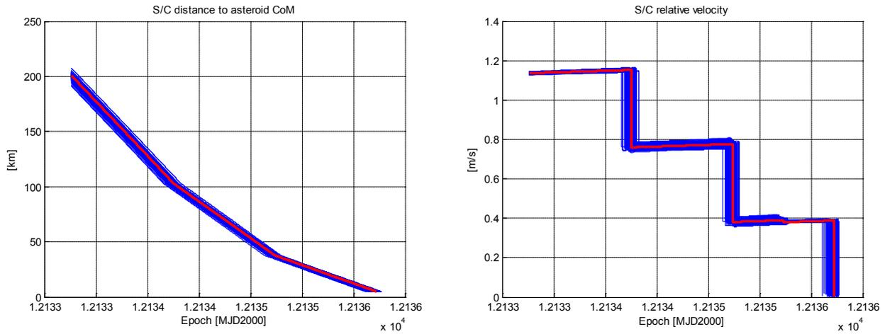
Figure 7: Close Approach distance (left) and relative velocity (right) to asteroid in Monte Carlo simulation
