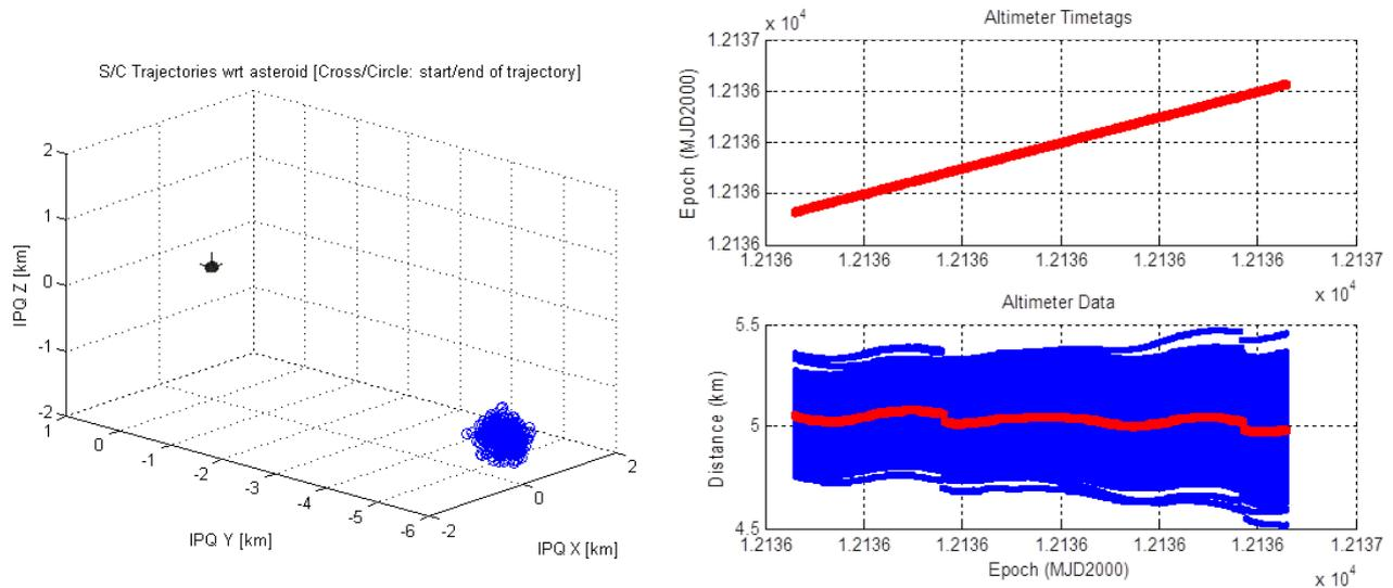
Figure 9: Arrival Inertial Hovering for 6h trajectories (left) and altimeter data (right) in Monte Carlo simulations
