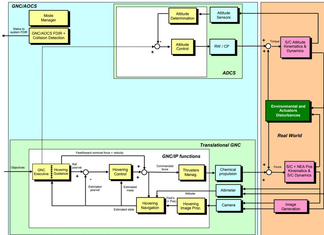
Figure 4: Functional architecture during Arrival Inertial for 6h (AIHM) and Body-Fixed Hovering (BFHM)
