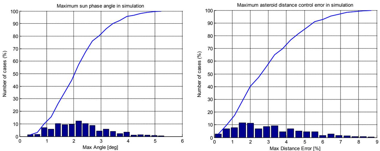
Figure 10: Arrival Inertial Hovering for 6h maximum sun phase angle (left) and maximum distance error (right) statistics in Monte Carlo simulations
