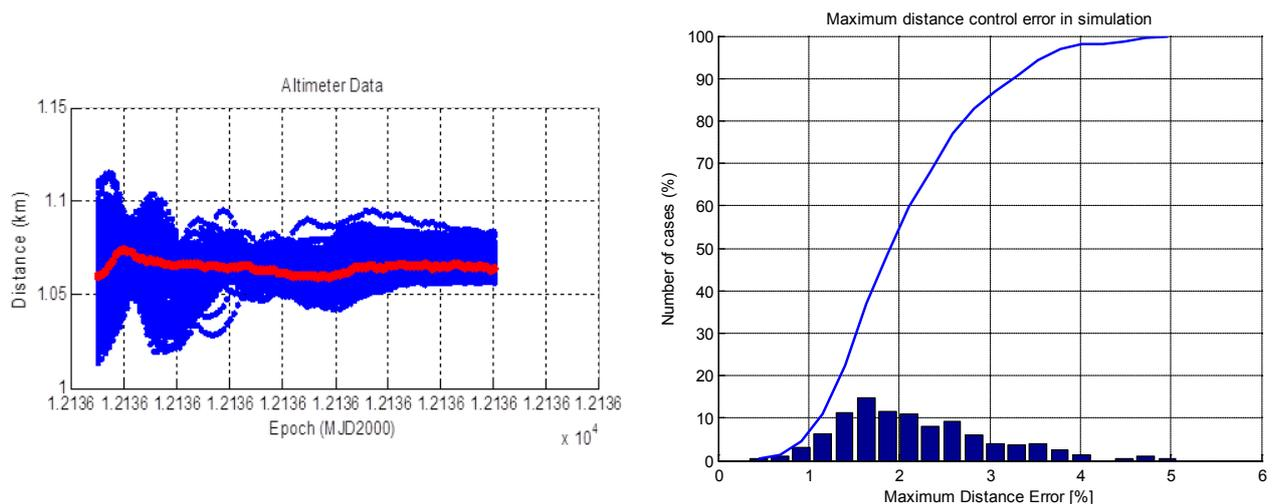
Figure 13: Body-Fixed Hovering altimeter data (left) and maximum distance error statistics (right) in Monte Carlo simulation
