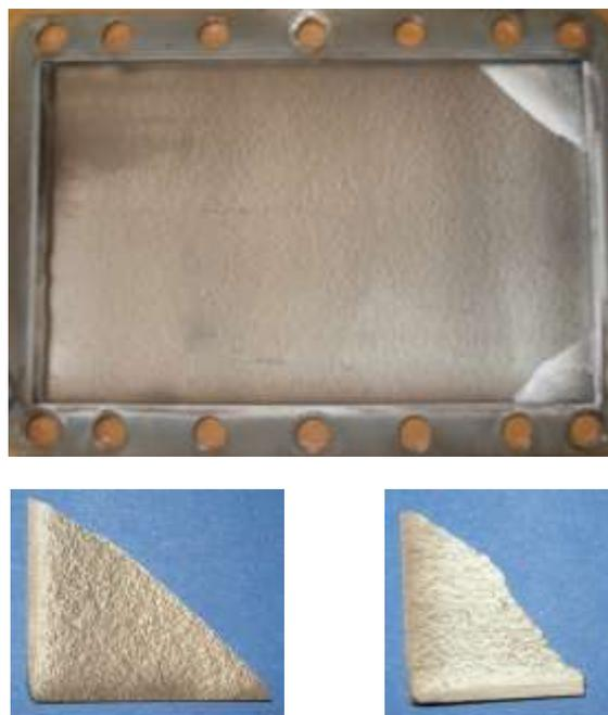
Figure 10: Titanium sample after high-temperature tests (small pieces were separated for analysis)
