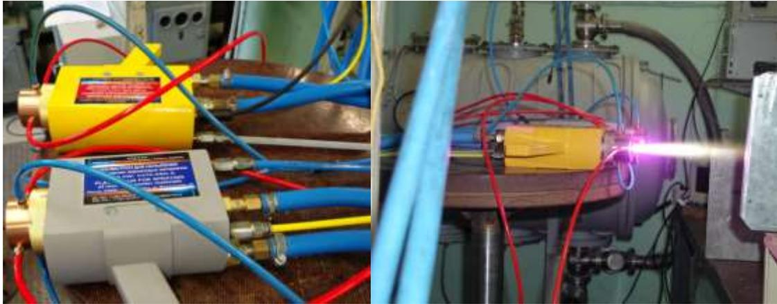
Figure 1: Electric arc plasma torches for deposition of metallic, intermetallic and ceramic powder materials
