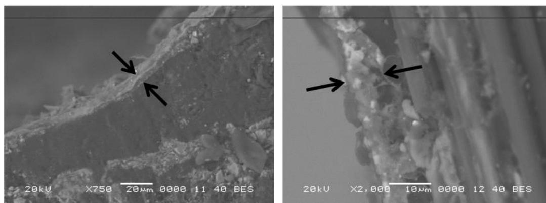
Figure 8: SEM coating cross section
