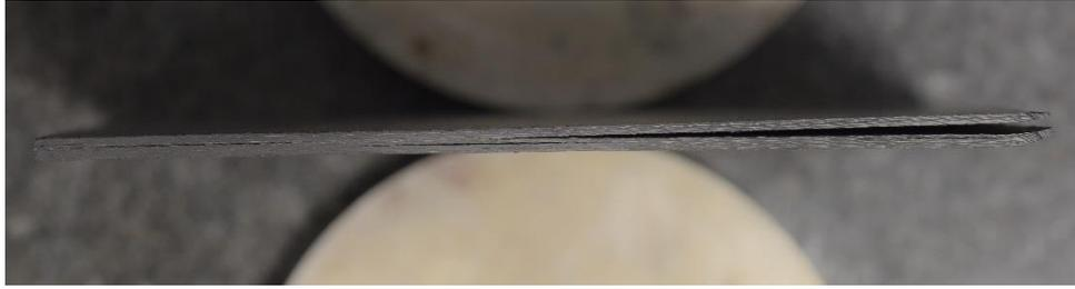
Figure 4: Severe delamination occurred during pyrolysis
