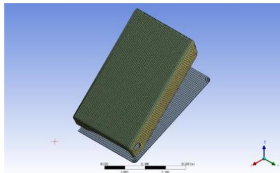
Figure 18: Finite Element Model 3D Mesh (half model)
