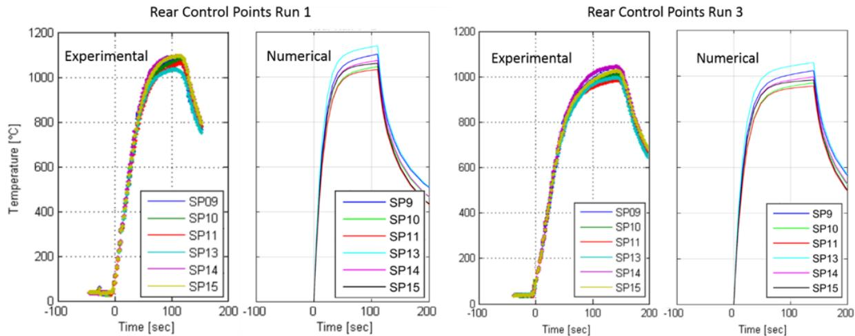
Figure 20: Experimental and numerical temperature variation at TC position for run 1(left) and run 3 (right)
