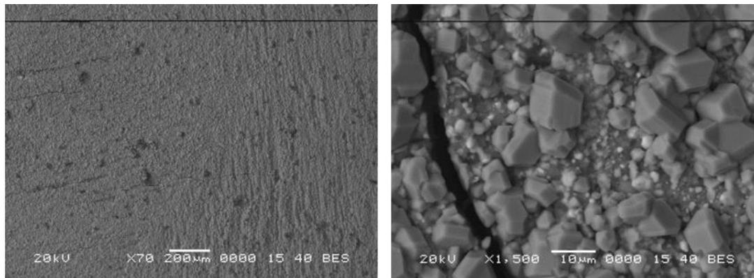
Figure 7: SEM of coated surface
