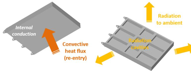
Figure 17: First thermal model on simplified geometry
