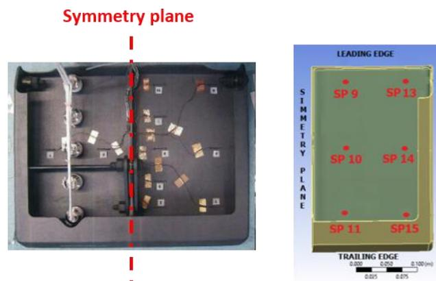
Figure 19: Thermocouples position on test article and on numerical model (half model)
