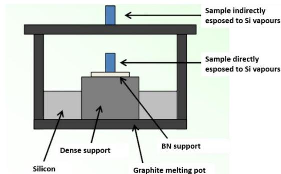
Figure 6: Coating deposition scheme
