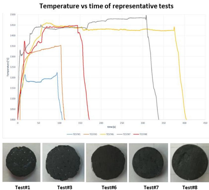
Figure 14: Temperature versus time of some representative tests
