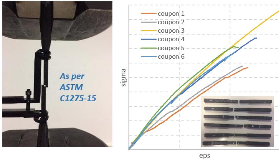
Figure 9: Tensile test
