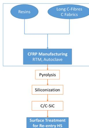
Figure 1: LSI manufacturing process
