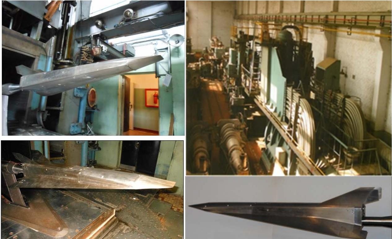
Figure 12: EFTV wind tunnel model and T-116 wind tunnel at TsAGI
