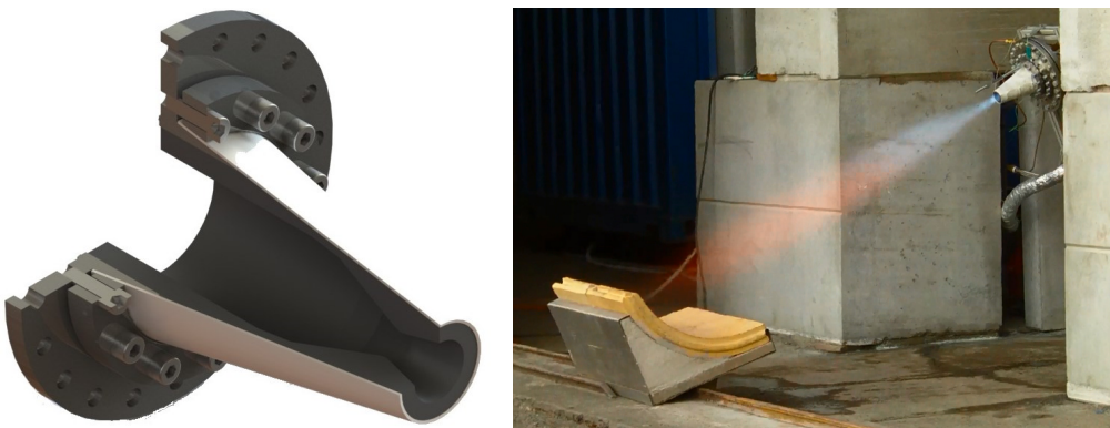
Figure 3: Test combustion chamber with OCMC corset
