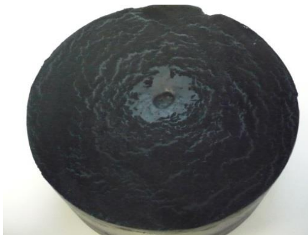
Figure 6: Fuel grain shape after the MHYCAS_17 firing test
