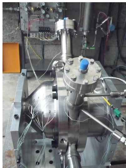
Figure 4: Thermocouples welded on the MHYCAS engine
