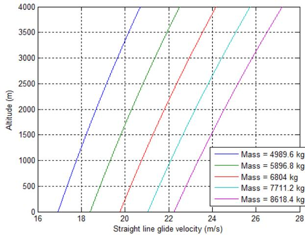
Figure 10: Parafoil glide velocity performance
