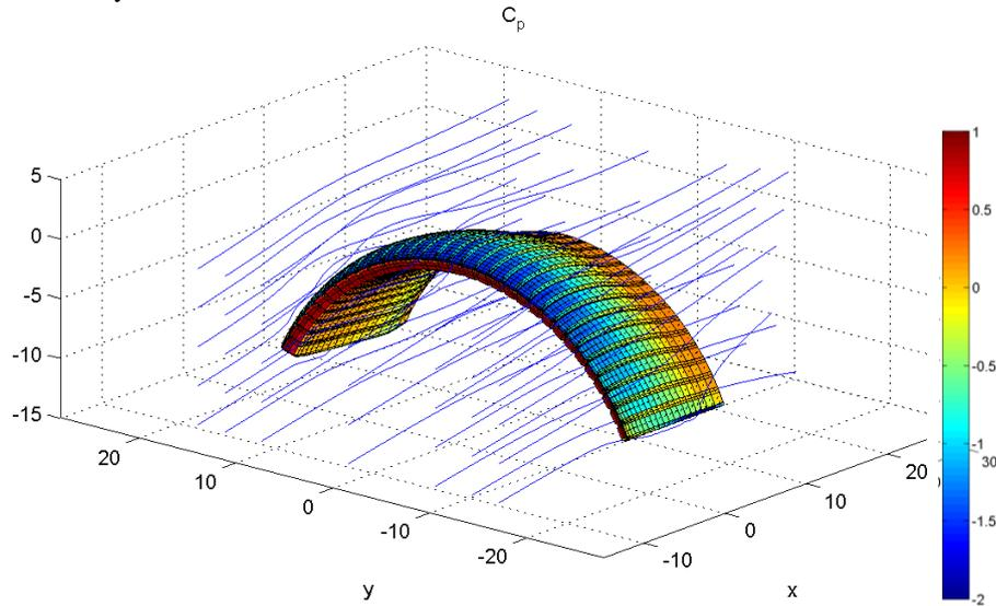
Figure 4: X-38 parafoil geometry, 3D Panel Method AoA=8.8 [deg]
