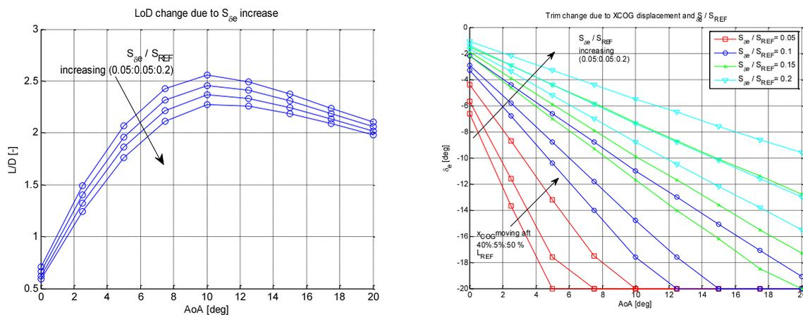
Figure 6: Elevator to reference Surface ratio effect and x coordinate of COG on trim and aerodynamics.
