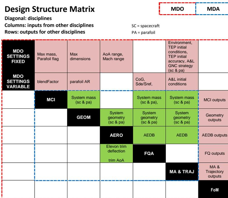
Figure 1: Design Structure Matrix (MDA and MDO) for REVLANSYS
