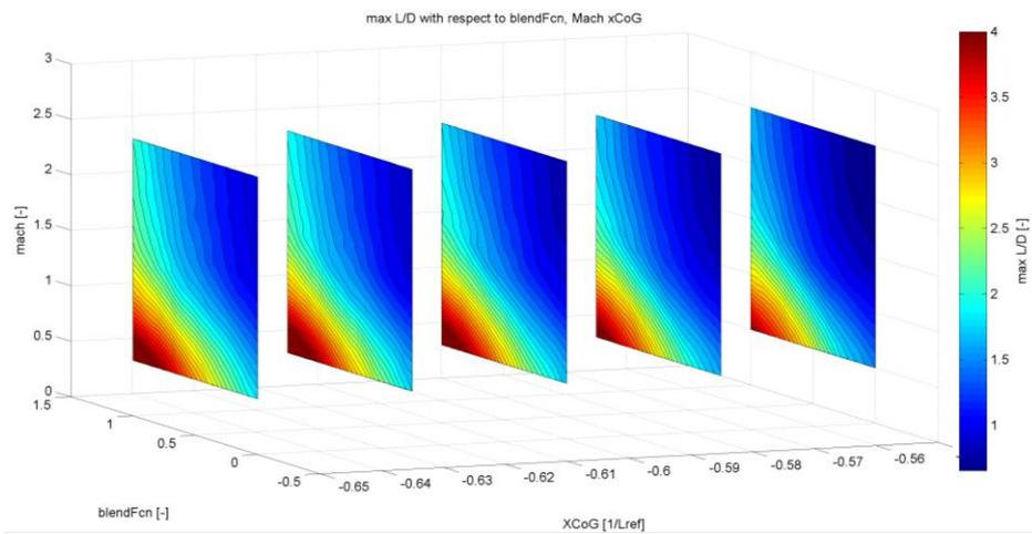
Figure 12: Max L/D with respect to XCoG, Blend function, and Mach.
