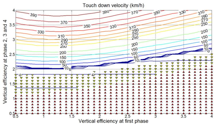
Figure 8: Touchdown velocity with respect to vertical efficiency (Horizontal Landing)
