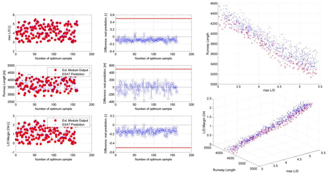
Figure 15: Horizontal landing. Max L/D, Runway Length and L/D margin: Pareto from metamodel and validation.
