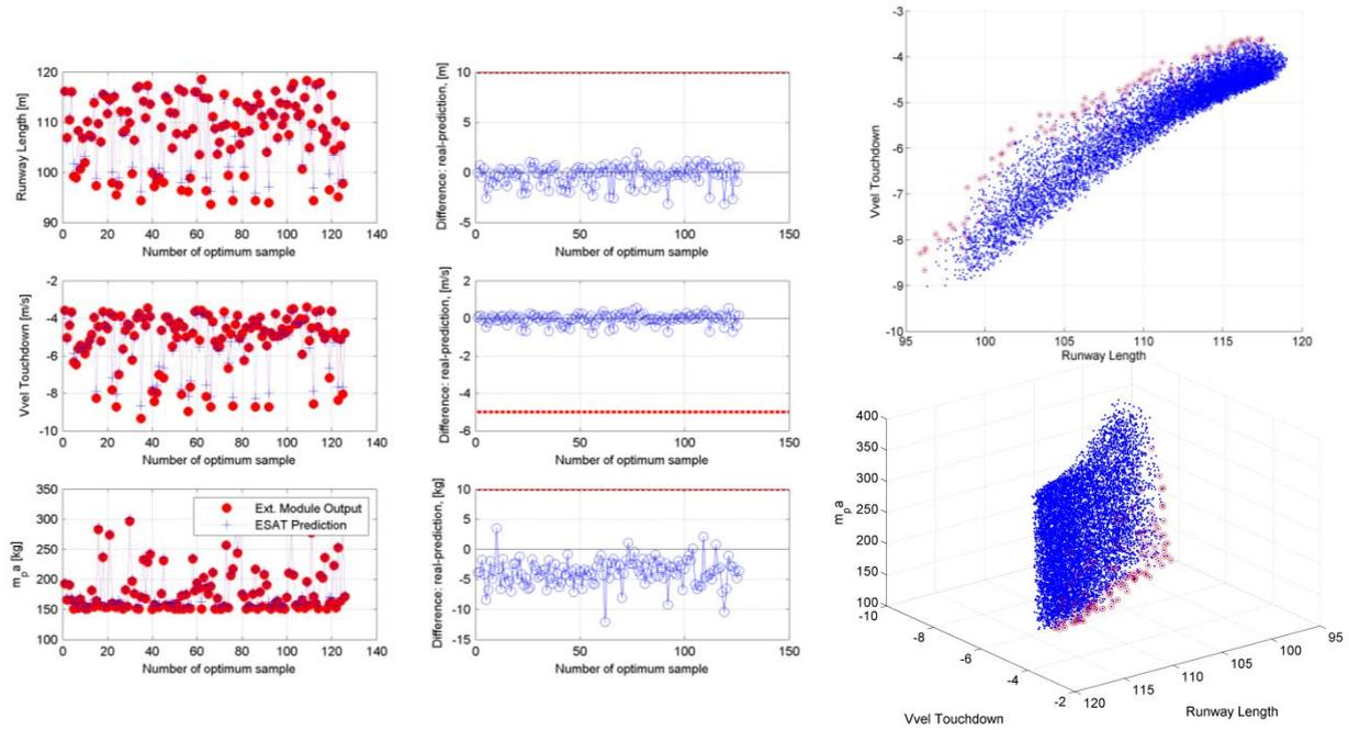
Figure 16: Soft landing. Runway Length, Vertical V and parafoil mass: Pareto from metamodel and validation.
