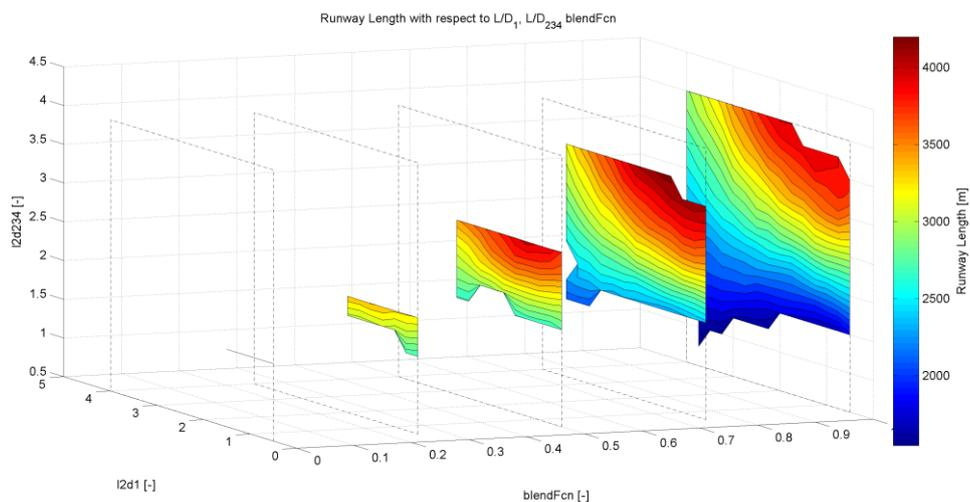
Figure 13: Runway length with respect to blend Function and  $L/D_1$ ,  $L/D_{234}$
