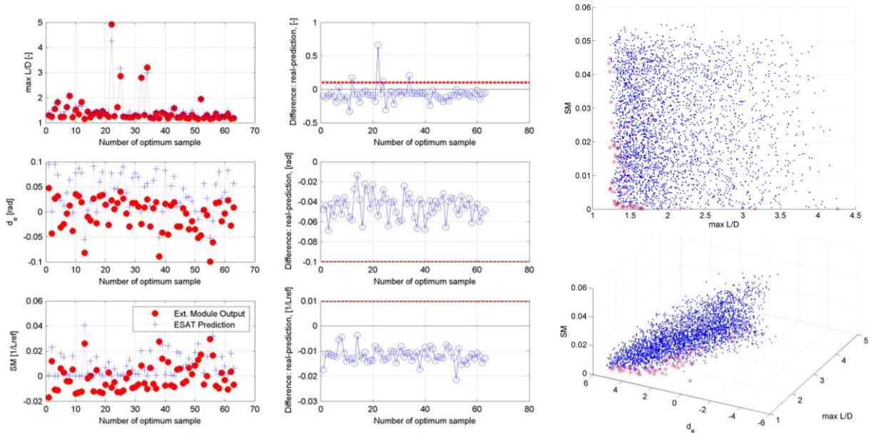
Figure 14: TAEM phase. Max L/D, Static Margin and elevator deflection: Pareto from metamodel and validation.
