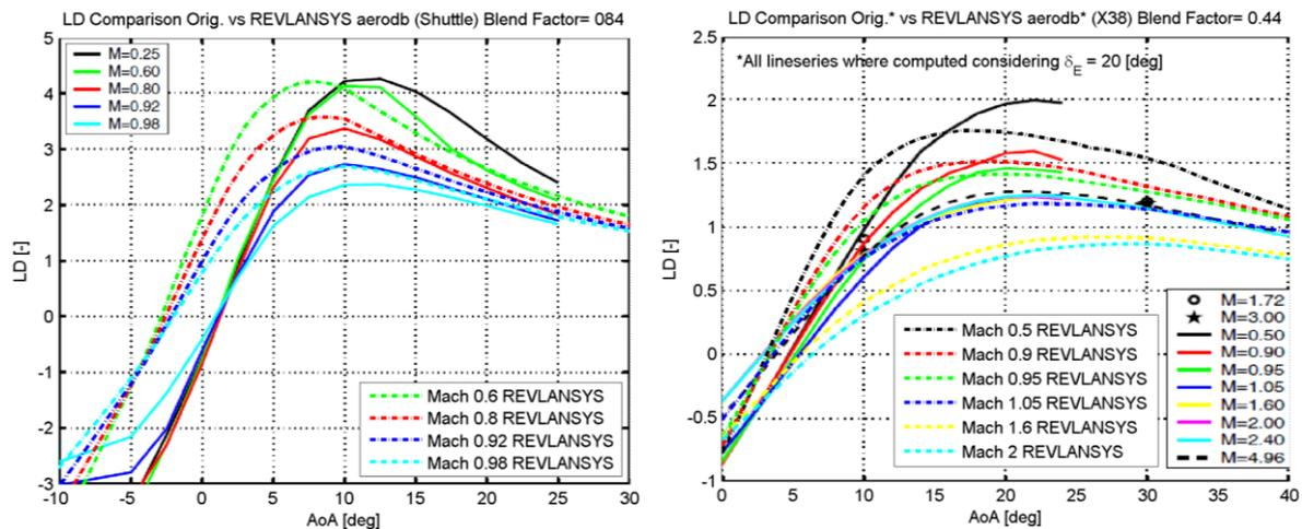
Figure 5: Shuttle (left), and X-38 (right) aerodynamic Database [1], compared to REVLANSYS Blend Function.
