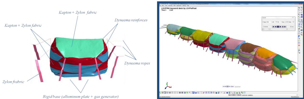
Figure 22: Baseline Concept, design solution and LS-Dyna thermo-structural simulation of bags inflation
