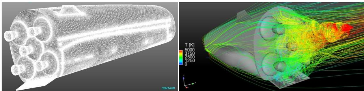
Figure 20 : Surface mesh of the computed vehicle (a) and T along streamlines (b)
