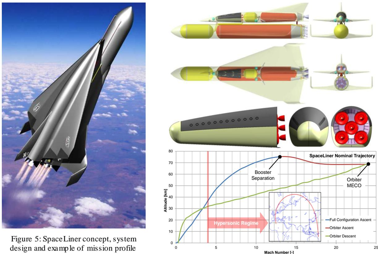
Figure 5: SpaceLiner concept, system design and example of mission profile
