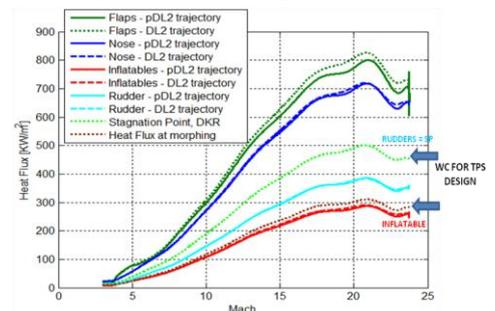
Figure 17: Heat flux sizing profiles
