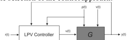
Figure 18: LPV controller scheme
