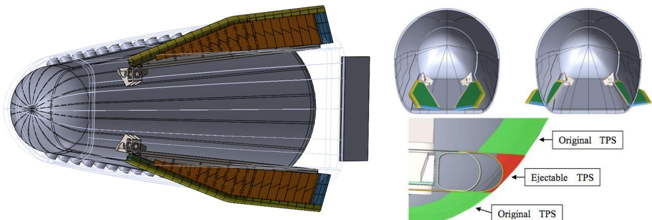
Figure 23: Backup Concept, mechanical and structural design
