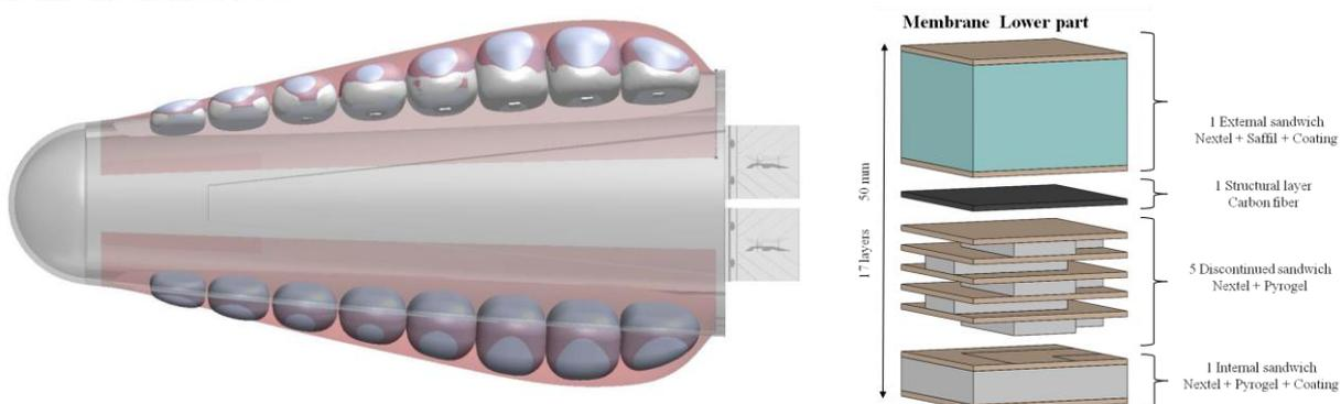
Figure 21: Baseline Concept, mechanical and structural design
