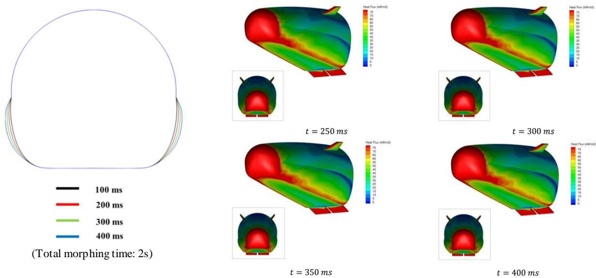
Figure 19 : Morphing geometry (a) Heat Flux time evolution (b) (200 – 400 ms)
