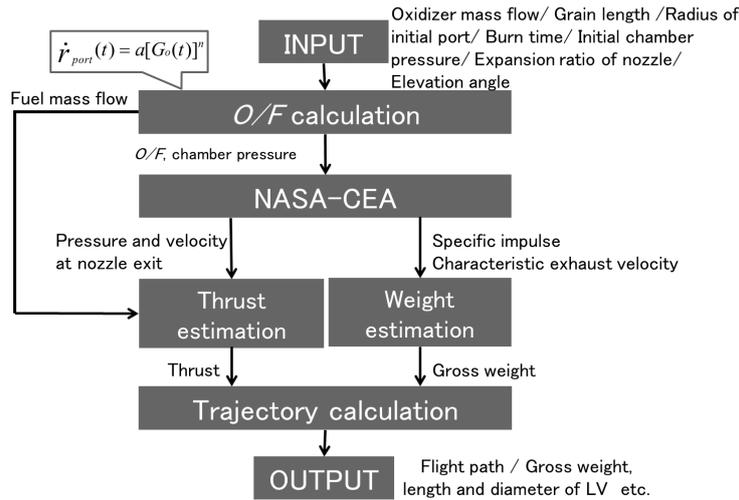
Figure 2: Evaluation procedure for HRE.
