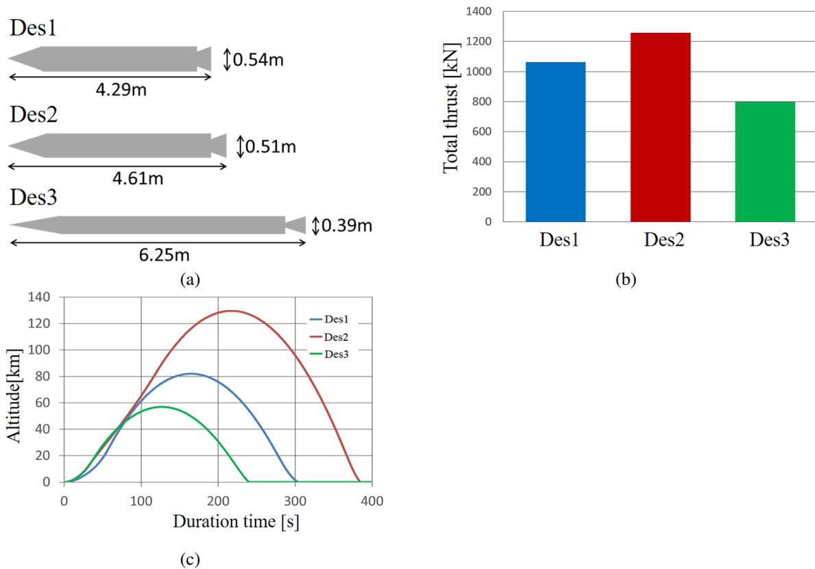
Figure 7: Comparison of designs based on the non-dominated solutions. (a) Designs of LV, (b) Thrusts of the HR under each design, and (c) Time history of the altitude for each design.
