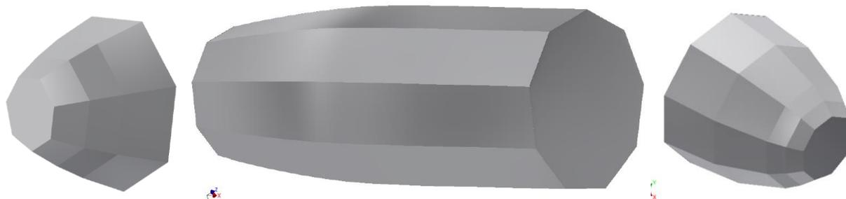
Figure 6 : Shapes of the gas cells: Rear, Middle, Front gas cell (from left to right)
