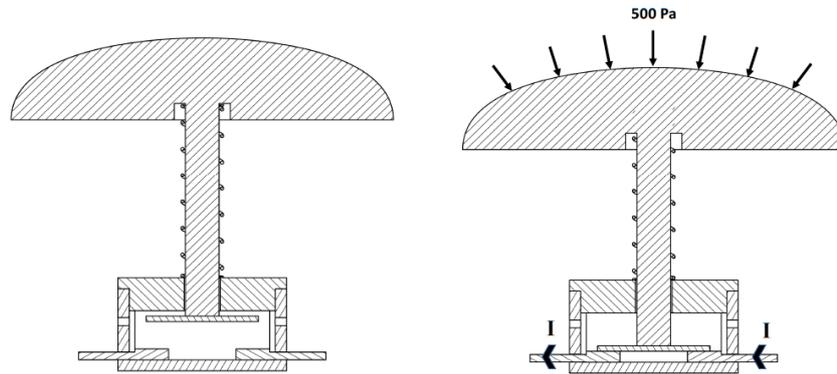
Figure 13: Working principle of the overpressure sensor
