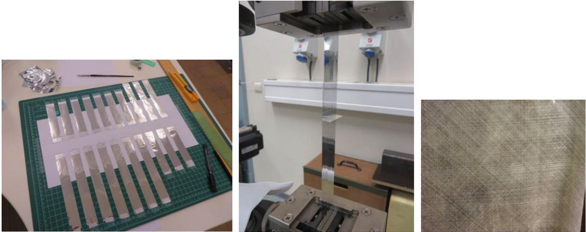
Figure 8: Samples cut for the tests (left), test of a side seam sample (middle), EVAL/Composite (right)
