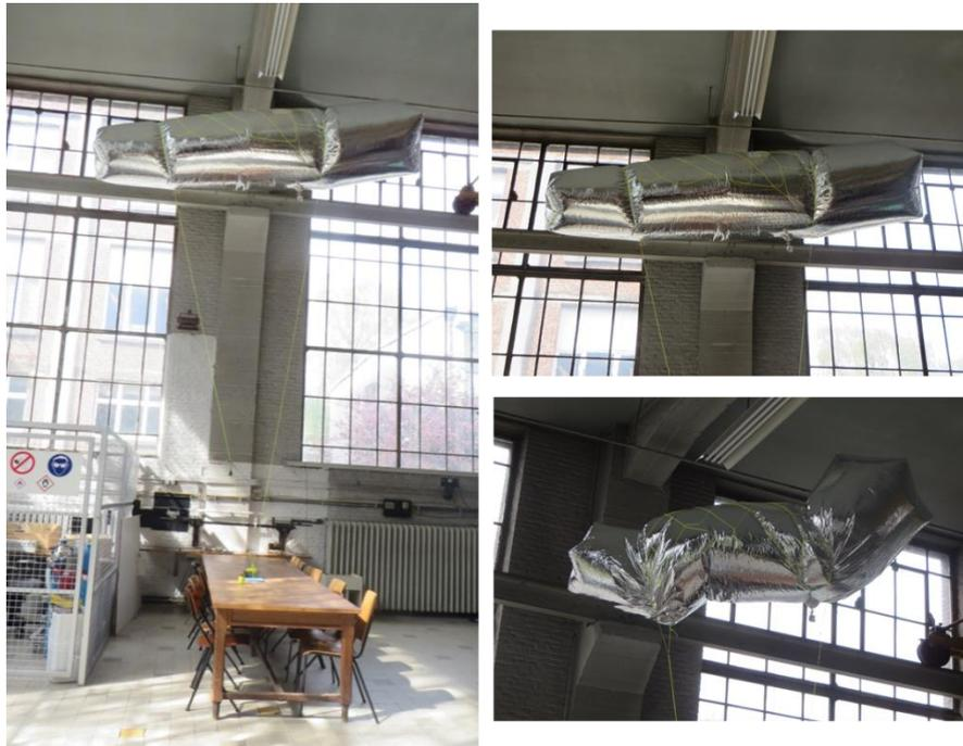
Figure 10 : Small balloon using lap seam. Leakage rate test
