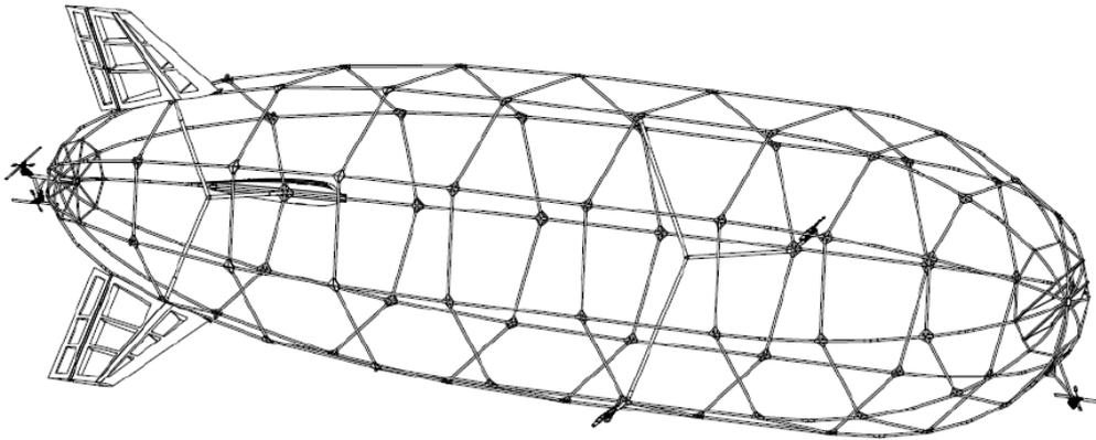
Figure 4: FlyWin Demonstrator rigid structure
