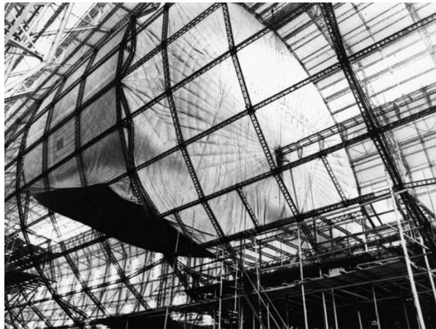
Figure 5: A partially inflated gas containing cell inside of the airship's structure [12]
