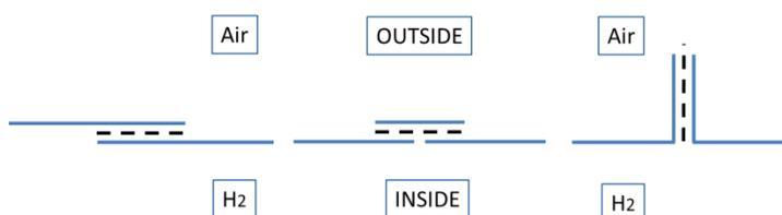
Figure 7: Joining techniques. Lap seam, Butt seam, Side seam (from left to right)
