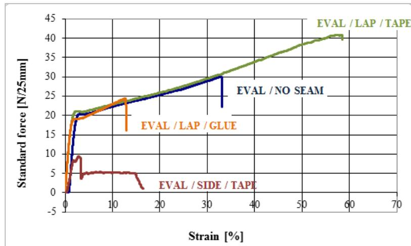
Figure 9: Typical curves of EVAL strength tests
