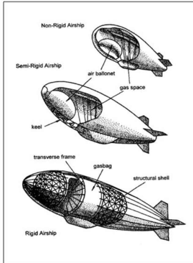
Figure 3: Structure design options for airships [10]
