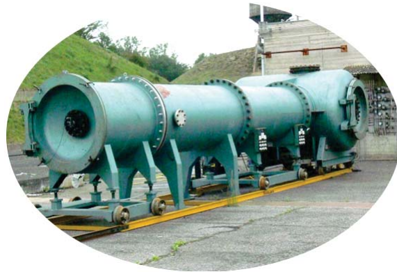
(b) 18 m 3 depressurized tank located at ONERA's Fauga center
