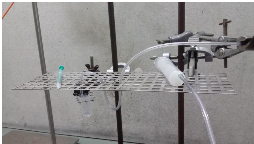
Figure 3 Experimental set-up to investigate hypergolic behavior of the investigated bi-propellants.
