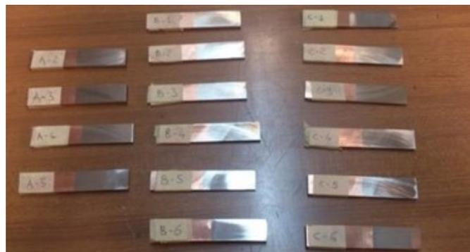
Figure 10 - CSM Brazed samples
